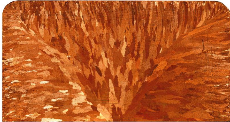
Figure 1. Crystalline copper; the illustration shows half of a slice through a copper ingot.
