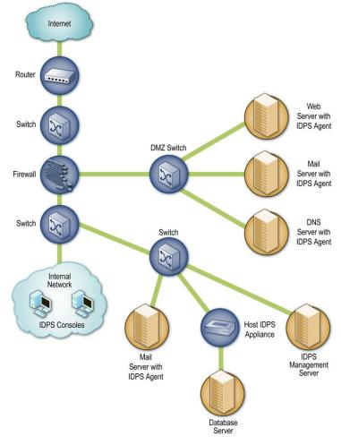
Figure 1: An example of how a hostbased IDS can be deployed [SM07, Figure 7-1]. Note 11 the IDS sensors/agents monitoring the web server, mail servers, Domain Name System server and database server; 22 a host-based IDS can exist in the form of software or hardware.
