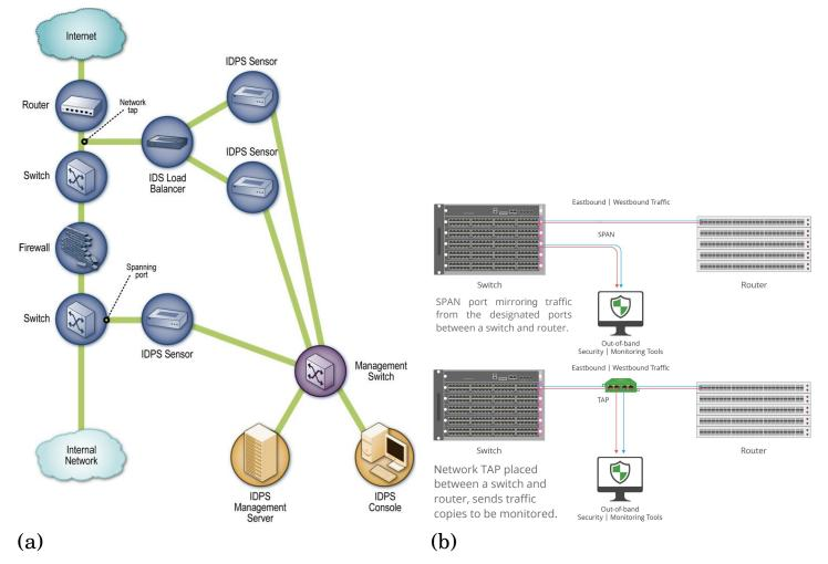
Figure 4: (a) An example of a passive network-based IDS [SM07, Figure 4-3]. (b) SPAN vs TAP for monitoring [Gar21].
