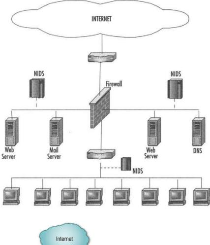
Figure 2: An example of how a network-based IDS can be deployed: two IDS sensors monitoring two public-facing subnets and one IDS sensor monitoring a subnet of internal terminals [BE07, Figure 1.1].
