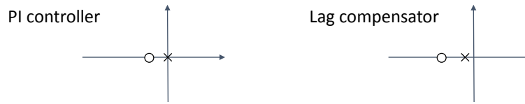
Figure 22: PI controller vs. lag compensator in terms of pole and zero.
