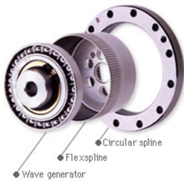
Figure 5: A harmonic drive consists of a circular spline, a flexispline, and an elliptical wave generator. The flexispline takes on the shape of the wave generator when the latter is inserted into it. Image source: https://www.hds.co.jp .
