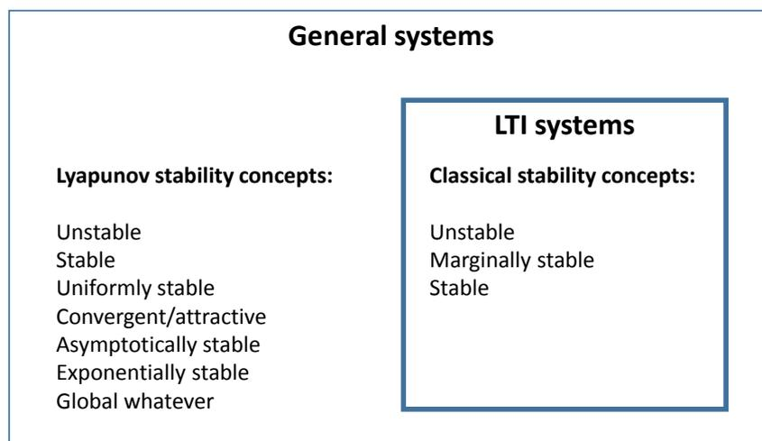
Figure 9: Keywords in the Lyapunov sense and keywords in the classical sense. A keyword in the classical sense can be mapped to multiple keywords in the Lyapunov sense.
