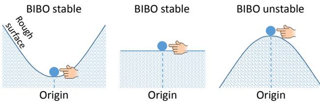
Figure 1: Analogies for external stability. Say the ball is at the origin, and we give the ball a poke of finite strength. Think of the distance between the ball and the origin as the forced response. If the ball eventually stops at a certain spot, the system is externally stable (BIBO stable). If the ball keeps moving away, the system is externally unstable (BIBO unstable).
