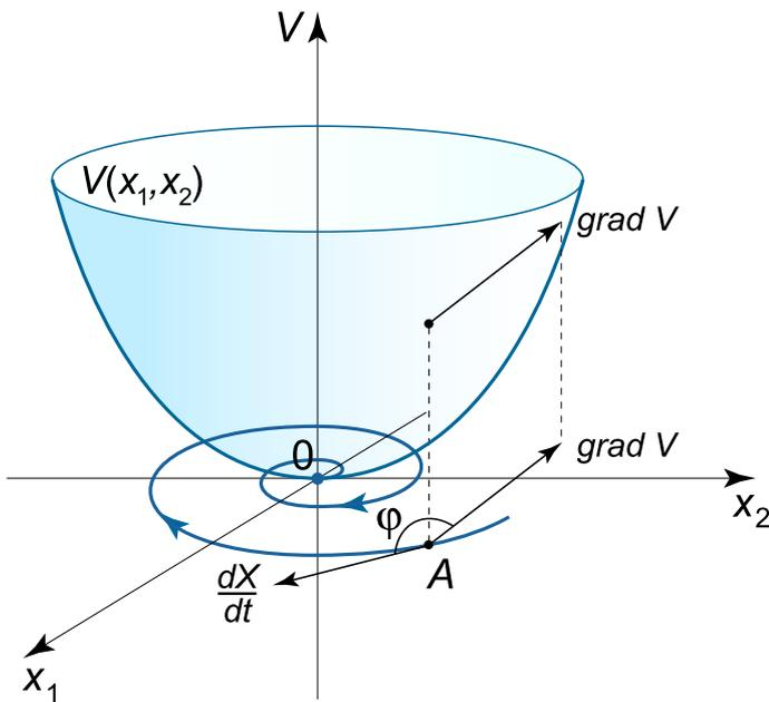
Figure 10: If the origin is stable, all system trajectories follow the direction of nonincreasing  $V$ , where  $V$  is the Lyapunov function.  $\dot{V}$  is exactly the inner product of  $\text{grad } V$  and  $\frac{dx}{dt}$  in the figure. Image source: <https://www.math24.net/wp-content/uploads/2016/09/lyapunov-function2.svg>
