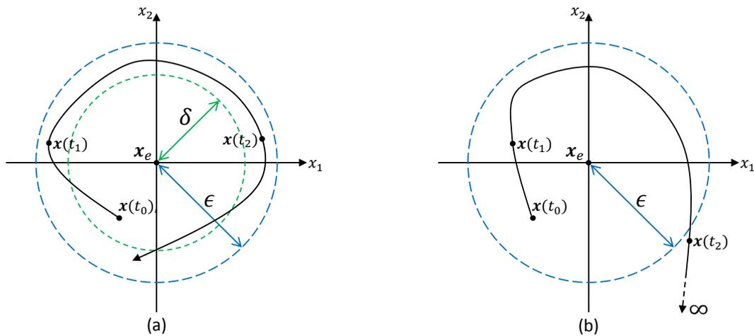
Figure 6: Examples of equilibria in a two-dimensional state space that are (a) Lyapunov stable, (b) unstable.
