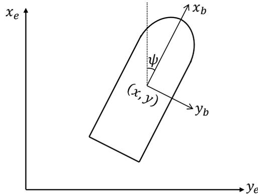
Figure 12: The position parameters of a ship:  $(x, y, \psi)$ . Notice the earth axes and body axes follow the north-east-down and front-right-down conventions respectively.
