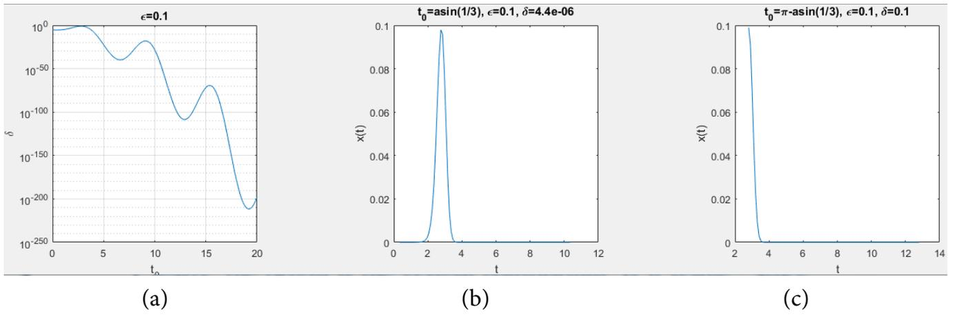
Figure 7: The origin of system (5) is not uniformly stable. (a) shows  $\delta$  generally decreases with  $t_0$ . (b) and (c) show  $x_0$  needs to be significantly closer to the origin for  $t_0 = \arcsin(1/3)$  than for  $t_0 = \pi - \arcsin(1/3)$ , given the same  $\epsilon$ .
