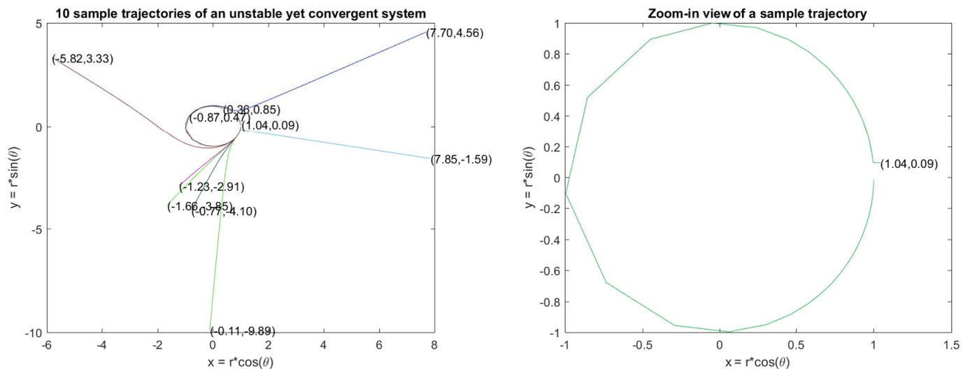
Figure 5: Phase portraits of system (1). The left figure shows 10 trajectories with a random initial state converge at the equilibrium point  $(1, 0)$ . The right figure shows an example of how a trajectory can start very close to the equilibrium point and yet make a sizeable excursion before reaching the equilibrium point. This is a classic example of how an equilibrium can be *unstable* and yet *convergent* (having all nontrivial trajectories converging to it).
