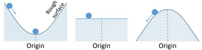
Figure 2: Analogies for internal stability. At  $t = 0$ , we place a ball at a random spot other than the origin, and see if the ball will settle at the origin (asymptotically stable), or settle at some point other than the origin (stable), or keep moving away from the origin (unstable). Think of the the distance between the ball and the origin as the natural response. Illustration inspired by [WL07, Figure 6.1].
