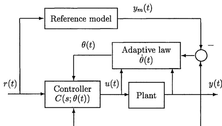
Figure 14: The direct model reference adaptive control system architecture [Tao03, Figure 1.4]. Here,  $\theta$  denotes a generic controller parameter.
