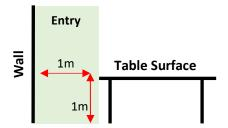
The entry system prototype must be able to account for people entering through the 1m wide, 1m high, gateway. However, physical devices like boom gates do not have to be to scale - they only need to demonstrate the functionality.
