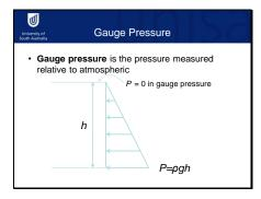
Okay, now a little bit of terminology. "Gauge pressure" is the pressure measured relative to atmosphere. According to gauge pressure, at the top of a body of water, the pressure is zero and it rises to pgh at the bottom.
