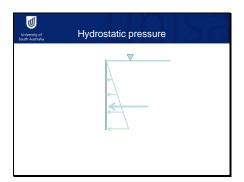
The distributed pressure is effectively a linearly increasing load, which is equivalent to single force acting through centroid of the pressure distribution.
