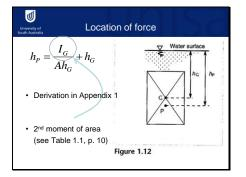
Here's the general equation we use to calculate the depth hP where the hydrostatic force will act on a submerged flat surface of any shape. You can find the derivation at the back of the textbook if you want to see where it comes from.
