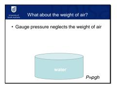
Gauge pressure neglects the weight of air. If we include the weight of the air sitting top of the water, that's known as "absolute pressure".
