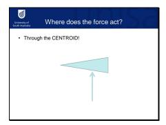
The force acts through the centroid, so to balance the wedge with a single support it'd need to be through the centroid too.
