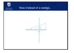
So now imagine a linearly-increasing (distributed) load supported by a single force acting at the centroid of the load distribution. This is just a sort of schematic version of the wedge.
