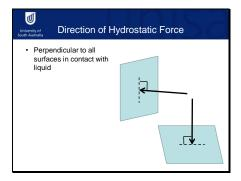
It's important to note that the hydrostatic force acts exactly perpendicular to the surface, irrespective of the orientation of the surface.
