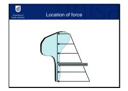
Actually, the location of the force depends on both the pressure distribution and the shape of the submerged object. Here's a totally arbitrary shape with a pressure distribution.
