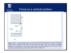
Figure 1.10 shows a vertical gate at the end of a sewer which discharges to a river. Hopefully this is discharging properly treated water so it doesn't pollute the river! Anyway, this is the sort of situation where you'd need to know the force acting on the gate to make sure you can actually open it properly.
