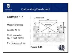
Here's a buoyancy example from the text book. We've got a pontoon 10 by 5 metres and 2 metres high, with a mass of 50 tonnes. It's floating stably in seawater so we know the buoyancy force has got to equal the weight. Note that the density of seawater is slightly higher than freshwater, which is usually about 1000 kg/m3. We need to work out how much water this pontoon is going to displace, and then use that to determine the depth of immersion and the freeboard.
