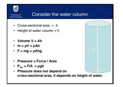
In hydrostatics, the force at a given depth is due to the weight of the water above.
