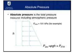
The absolute pressure distribution in a water body is similar to gauge pressure, it's just the addition of constant atmospheric pressure (about 101 KPa) all the way down.
