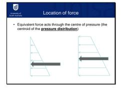
So our equivalent force acts through the centre of pressure (the centroid of the pressure distribution). Two different examples of pressure distributions are shown here.
