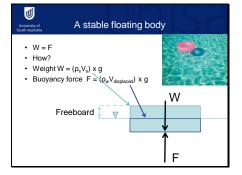
If the weight of a floating body equals the buoyancy force, it'll be stable. We see things floating in water every day. How do the forces balance?
