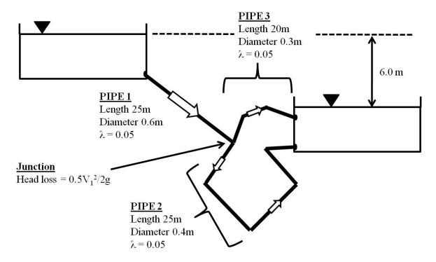
The discharge rates in all 3 pipelines are unknown. Your task is to complete the hydraulic analysis up to the point of obtaining 3 equations for the three pipe velocities. You must include friction and minor losses in your analysis. <u>Simplify the equations as much as possible</u>, but **you do not have to solve the three equations**.
