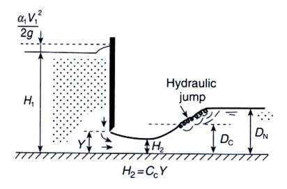
(a) Using the chart below and iteration (if necessary), determine the height Y at which the gate should be set to give an upstream depth  $(H_1)$  of 3.25m.
