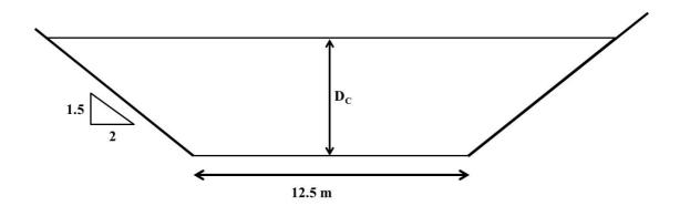
The critical water depth  $D_{\text{C}}$  on the channel centreline is known to be between 0.65 and 0.75 m.
