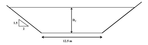
The critical water depth  $D_c$  on the channel centreline is known to be between 0.65 and 0.75 m.
