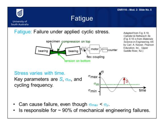
Fatigue is the failure of a material or component under an applied cyclic stress. It is a form of failure that occurs most often in dynamic structures. Structures that are experiencing dynamic and changing stresses. Examples of these kinds of structures are bridges, axels in vehicles, elevator cables and airplane components. The stress experienced by the material varies with time but it may be uniaxial tension or compression, flexural or torsional.
