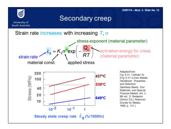
To calculate n you need to plot the logarithm of the steady state creep strain rate against the applied stress. This yields a straight line with a gradient of n. It is also clear that this changes with the experimental temperature.
