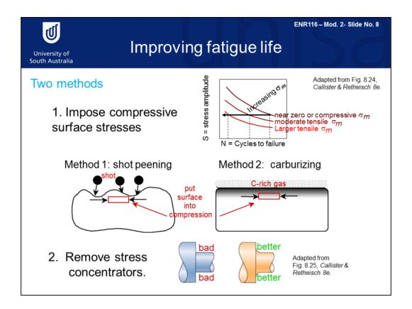
There are two main methods to improve the resistance of a material to fatigue. The first of these is to introduce compressive stress into the surface of the material to suppress crack growth.
