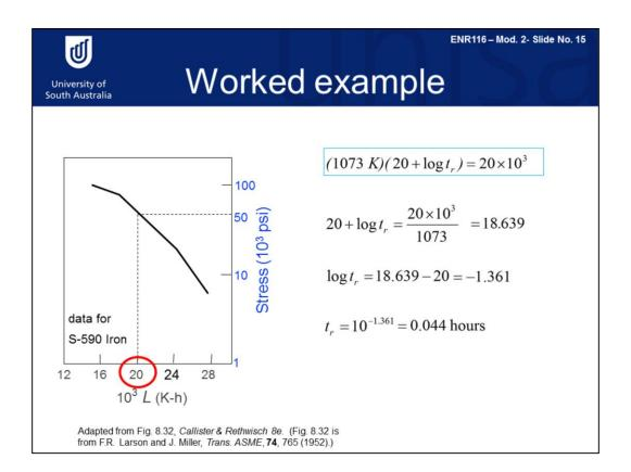
We can calculate L by using the data provided and the graph and we can see that The Larson-Miller parameter is 20,000. 800°C is equal to 1073K. Therefore 20+log t<sub>r</sub> multiplied by the temperature in Kelvin is equal to 20,000.
