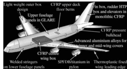
Figure 2. Metal/fiber applications in A380 airplane from Airbus 45 . Mat. Res. vol.9 no.3 2006
