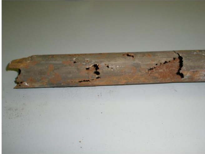
Mild steel heat exchanger tube exposed to caustic
