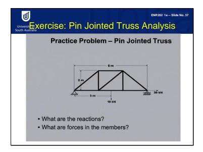
Here is another example. This is a truss problem with pinned supports on the left side and a roller support on right side. For the truss member or for truss structure, you have to calculate reaction forces, and also forces inside the truss members. Pause the presentation and try to work these out now. The solution is on the next six slides.
