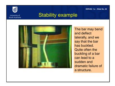
In this example, we have a column, and if we apply loadings on the column (apply compression on the column), it will become shorter and shorter. But if the column is very thin and you apply the compression, it will suddenly buckle, so the straight column will change its shape to a curved column. We call this phenomenon buckling. You have to use stability analysis to stop buckling in the column.
