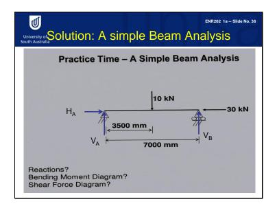
We have three equilibrium equations, two in forces and one in moment, for one object. All forces in a vertical direction are zero. That means sigma V equals zero, because we have a symmetric structure and symmetric loading. VA equals VB equals 5Kilo Newtons. All forces in a horizontal direction are zero. That means sigma H equals zero, HA equals 30Kilo Newtons. Take moments about the A point. All moments together are zero, which means that these calculations are correct.
