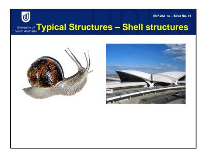
On the left you can see a natural shell structure. We use the theory behind this natural structure to build long span structures, particularly roof structures, in this kind of shell structure.
