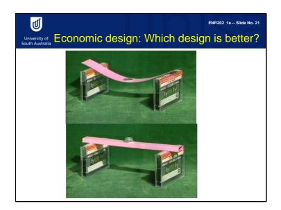
In design, you have to consider cost. For example, this is an example of beam design. We are using the same material for both designs. In the top image, the beam can carry only one coin. However, if you use the same material, but change the cross section and the shape of the beam, it can carry several coins. As we can see, the bottom design is more economic than the top design. This is an example of using mechanics theory to produce economic design.
