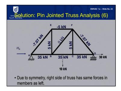
Due to symmetry, the right side of the truss has the same forces in members as the left. Finally, we work out that the truss members forces altogether look something like this.
