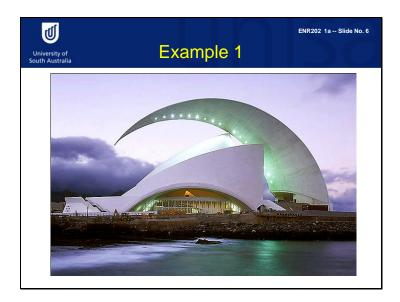
This is a long span building, with a large span roof. In fact, the roof is the kind of structure in which we might have acting loads : for example, wind load and snow load acting in the middle. So the loads on the roof have to be transferred to the foundation.
