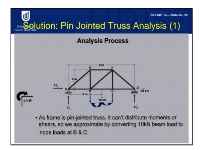
What are the reaction forces here? Just separate the 10 kilo Newtons into two parts, with the first 5 kilo Newtons on point B, and the other 5 kilo Newtons on point C. Try to work out the vertical reaction force at point A (VA), the horizontal reaction force at point A (HA), and the vertical reaction force at point D (VD).
