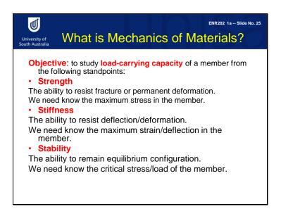
Lets come back to the introduction of the unit: What is mechanics of Materials? The objective of this unit is to study load-carrying capacity of a structural member from following three standpoints: Strength, stiffness, and stability.
