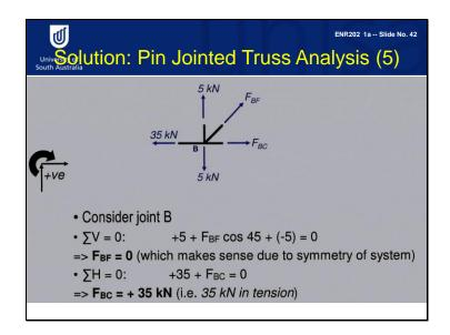
Now we come to the B joint with one known force and 2 unknown forces. We now consider equilibrium equations of the joint. For this joint, we have 2 equilibrium equations, which means all forces in horizontal direction and vertical direction are zero, so we have member force in BF is 0KN means no force, and remember horizontal forces, so force in member in BC is 35KN means tension.
