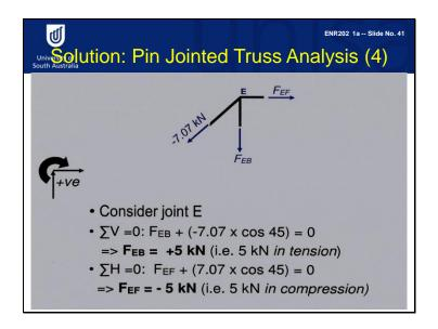
Now we come to the E joint, with one known force and 2 unknown forces, and we consider equilibrium equations of that joint. We have 2 equilibrium equations, that means all forces in the horizontal direction and vertical direction are zero, so we have member force in EB is 5KN means tension, and remember horizontal forces, so force in member in EF is negative 5KN, which means compression.
