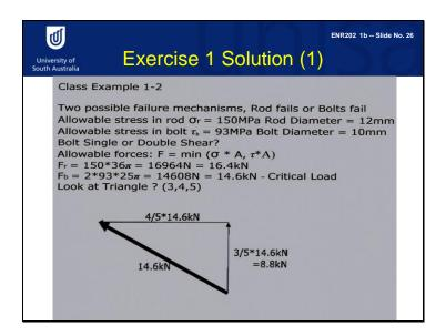
For the solution, you have to calculate the maximum load the rod can carry, the maximum load the bolt can carry.
