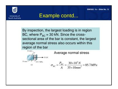
So, the maximum average normal stress is equal to 30 Kilo Newtons divided by the area of cross section. Convert force Kilo Newtons into Newtons. The area of the cross section is 35 mmms times 10 mms, which is equal to 350 square mms. That is 85.7 Newtons per square mm (also called Mega Pascals).
