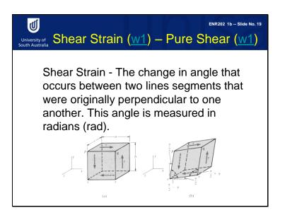
Shear strain occurs due to shear force. The shear force will cause the object to change in angle, resulting in shear strain. Shear strain is measured in radians.
