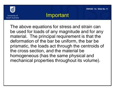
The equations for stress and strain can be used for loadings of any magnitude and any material. The principal requirement is that deformation of the bar is uniform. The bar should be straight and have a constant cross section throughout its length. The loadings act at centroid of the cross section. The material is also uniform.
