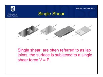
In this example, the connection of the bolt is resisted by the external force at only one shearing area. So we called this a single shear.
