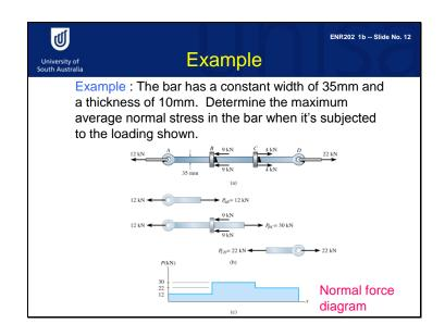
In this example, we have a bar with different parts. We have a load acting at point A of 12 Kilo Newtons, a load acting at point B which is altogether 18 Kilo Newtons, a load acting at point C which is altogether 8 Kilo Newtons, and a load acting at point D of 22 Kilo Newtons. The cross section of the bar is 35 millimeters in width and 10 millimeters in thickness. We want to calculate the maximum normal average stress in a bar.
