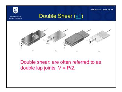
In this connection, the middle plate is subjected to force P, and the top and bottom plates are acting at half force P. We cut the bolt between the top and middle plates, and the bottom and middle plates cross section. Then, we analyse the middle plate with two shearing surfaces on the bolt. Total force is P shared by both shearing surfaces by half force P. So, this connection is a double shear. In figure C, the plates are joined by glue.
