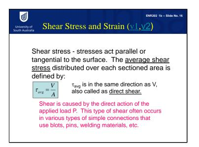
The Shear stress which is acting parallel to the cutting surface is equal to the shear force divided by the cutting surface area, called the average shear stress. It is denoted by the symbol *tou* acting in the same direction as shear force V.
