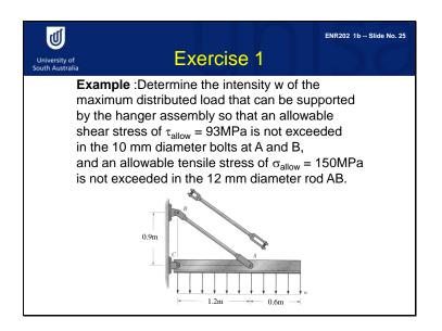
In this example, we have a beam and a hanger bolted at joint A. The bolt allowable shear stress is equal to 93 Mega Pascals. The bolt diameter is10 mms, and hangar allowable tensile stress is 150 Mega Pascals. The diameter of rod AB is 12 mms, and we need to calculate how much load can be applied on the beam. That means we just want to know the maximum uniform distributed load 'w'. That is maximum load acting on the beam.
