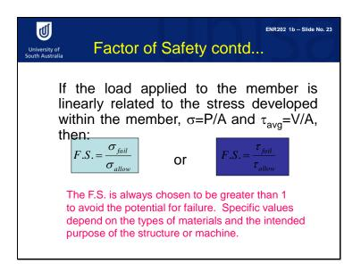
The factor of safety may also be defined based on maximum stress and allowable stress. That means that some kinds of material have failure stress or ultimate stress, which we know from an experimental test. We know that allowable stress is equal to failure stress divided by the factor of safety. Of course, the safety factor will be larger than one. We have another factor of safety related to shear stress, and this safety factor is equal to failure shear stress divided by allowable shear stress.
