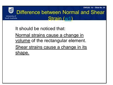
The difference between normal strain and shear strain is that normal strain causes a change in the volume of the object. For example, if we have tension, the bar gets longer and longer. However, shear strain only changes the shape, only changes the angle. There is no change in volume of the object due to shear strain.
