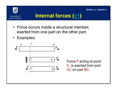
In this example, we have a bar subjected a force P acting at point A and another force in the equal and opposite direction at point B, as shown in the figure. I repeat one more time that the two forces are equal and are in opposite directions, so they create a balanced force system, and all parts of the bar will be in equilibrium.
