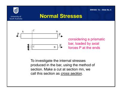
We now know the internal force acting at C. If we cut the section at C point that is perpendicular to axis of the bar, we say it is the C cross section. We call the intensity of the internal force over the cross section 'stress'.
