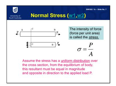
We use sigma to denote the stress. The intensity of the force means force per unit area. It is equal to P divided by A, because the total internal force acting at C is P. You use P divided by A to get the intensity of the force – that is, the stress.
