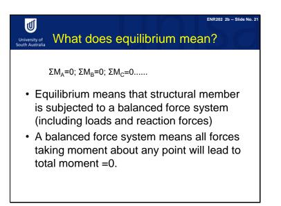
So, we have zero moment about A, and we have zero moment about B, and we have zero moment about C. The real meaning of equilibrium is that a structural member is subjected to a balanced system, and this balanced system will produce zero moment about any point.
