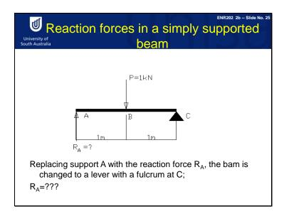
Right, let's replace the A support with a reaction force RA and a lever at Point C. What is RA? The answer is 0.5 KN
