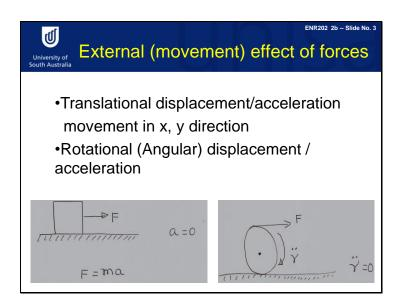
Firstly, let's have look at the external effects of forces. When we apply external forces on objects, we have movement. The first possible effect we can have is translational displacement or acceleration, calculated by Newtons law (Force equals mass times acceleration). This translational effect can be horizontal or vertical.
