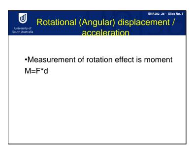
For rotational displacement, we first consider the measurement of rotation effect, and we use moment for rotational effect.
