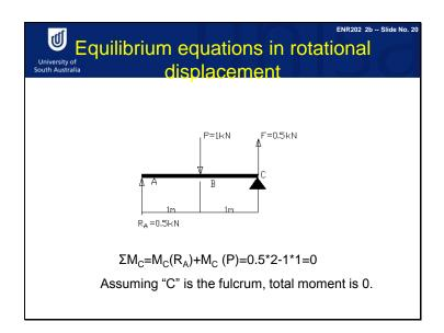
Now let's consider Point C as the lever. In this case, the RA force has moment about Point C equal to 0.5KN times 2m, or 1kNm. The P load has moment about Point C equal to 1KN times 1m, or 1KNm anti-clockwise. Therefore, we still have zero total moment.
