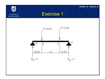
Here's another example. How do you calculate the reaction forces RA and RD here? Pause the presentation and try to work this out. The solution is on the next slide.
