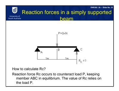
Let's look at another example, If we have a simply supported beam, and a load acting on middle span of the beam, we know this beam is in equilibrium. How do we solve the reaction forces at Point C? The reaction forces at C, together with the P load, together with the A support, will keep the beam in equilibrium, and the value of RC depends on the load P.
