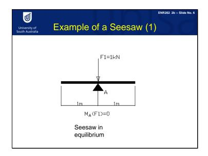
Let's look at a simple example: a seesaw. If Point A is the pivot of the seesaw, and we apply a 1 KN load vertically at A, the seesaw is still static. The equilibrium is not affected, even though we have an external loading on the seesaw.
