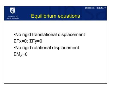
So the condition required for non-rotational displacement is that all moment together adds up to zero. This is the equilibrium equation of our object.
