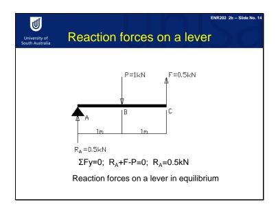
Lets look at the reaction forces on the lever. Some reaction forces are acting at Point A. Because the P load is acting down, and the F force is acting up, and these two forces together equal 0.5 kN down. But the lever is in equilibrium and will not move down. That means the total force acting on the lever should be equal to zero. That means RA is equal to 0.5kN. The forces acting on the lever here are RA (0.5kN up), P (1kN down), and F (0.5kN up).
