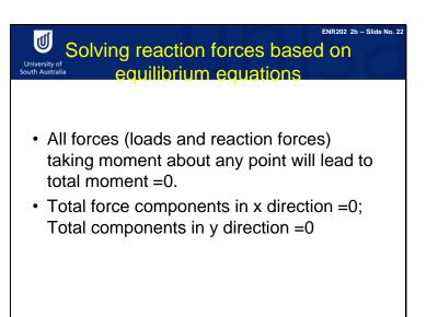
Now let's look at the general procedure. All forces, including loads and reaction forces, taking moment about any point will lead to a total moment of zero. All force components in x-direction together equal to zero, and total components in y-direction equal to zero. This is what equilibrium equations are all about.
