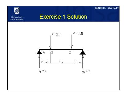
If we replace the support A by the RA, and we consider the Point D as a pivot, how many moments are acting on the pivot? The answer is 3 moments: one is 0.5KNm in anti-clockwise direction, another moment is 1.5KNm in anti-clockwise direction, and final moment is RA by 2 and this is in clockwise direction. The 3 moments together equal zero (0.5 plus 1.5 minus 2RA equals 0.) RA must be 1KN.
