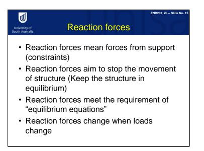
Reaction force is the force from support. For example, in the previous example we saw support A pivot forces acting on the lever, so RA was the reaction force. The reaction force aims to stop the movement of the structure.
