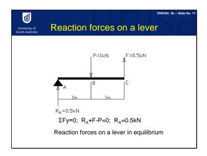
Let's come back to the lever reaction forces. We already calculated that RA is acting at Point A. The force acting at Point A is 0.5KN, the force acting at Point B is 1kN down, and the force acting at Point C is 0.5kN upwards.
