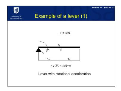
Let's look at another example ... a lever. Suppose we have a lever, and Point A point is the pivot of the lever. We apply an external load of 1KN to P at Point B. The distance between Point A and Point B is 1m, and we know the P load has a moment about point A equal to 1KNm. Because we have an unbalanced moment acting on the lever, the lever rotates clock-wise.
