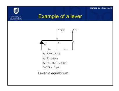
To stop the lever rotating clock-wisely, we have to apply another force on the lever. For example, if we apply a load at Point C, how much force do we need to stop the rotation of the lever? The answer is on the slide. To stop the rotation, the total moment acting on the lever must be zero.
