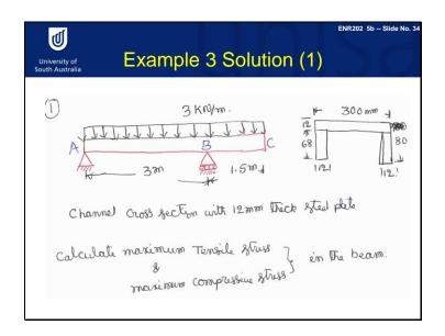
This overhang beam has a channel cross section of 300 millimeters by 12 millimeters, 68 millimeters by 12 millimeters, and another 68 millimeters by 12 millimeters, as shown in the figure.
