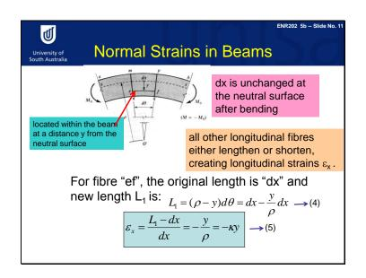
If we have normal strain in a beam after deformation, the beam changes into a curve. The O dash is the centre of the circle, as shown in the figure. Rho is the radius of the circular curve. We can say that for e-f, the original length is dx (that is, the original length before bending), and the deformed length (that is, the length after bending) is equal to rho minus y. That is the distance between the neutral axis and the e-f line multiplied by 'd theta'.
