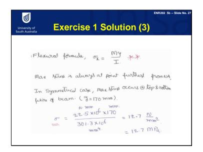
Use the flexure formula to calculate normal stress, which is equal to a bending moment of M times y divided by I.
