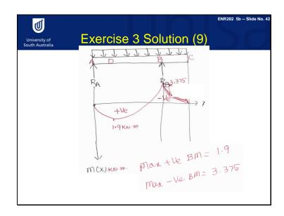
Connect all the bending moment values at important points, and we get the bending moment diagrams shown in the figure. You should try to draw the bending moment diagram on your own and check it against this figure.
