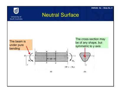
As shown in the figure, before the deformation we have a straight beam. The cross sections m-n and p-q located at distance 'dx' are also straight lines, as shown in figure a. Here, we consider the symmetry cross section about the y-y axis, as shown in figure b. We applied pure bending with negative bending moment 'Mo'.
