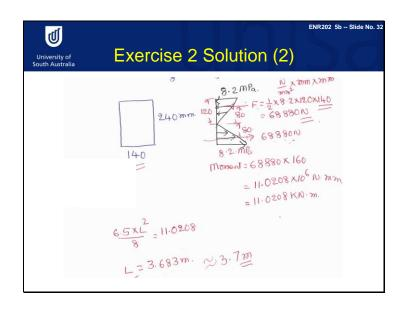
In positive bending moment, we have the top part of the beam in compression and the bottom part of the beam in tension, as shown in the normal stress distribution diagram. We have maximum compressive and tensile normal stress 8.2 Mega Pascals, as shown in the figure.
