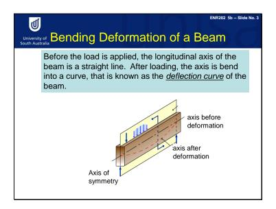
Beam bending refers to the application of vertical forces on a beam. Before force is applied, the beam is in a straight line. After applying the loads, the straight axis deforms into a curve. This deformation is known as bending.
