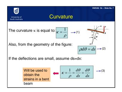
The relationship between curvature, which we denote as kappa and rho, is as follows: kappa is equal to 1 divided by rho, as shown in the equation 1. From the geometry of the figure, we can see that the radius 'rho' and the centre of the curve is O dash. The distance between m1 and m2 is 'ds' which is equal to rho times 'd theta', as shown in the equation 2.
