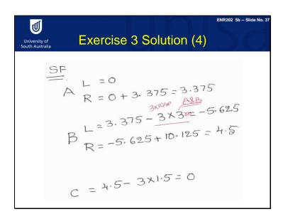
You now need to calculate shear force values at important points (check lecture 4b, slide 31 if you need to). We have three important points. The first is at the beginning of the UDL. The second is a supporting point, B. The third is another supporting point, C, which is at the end of the uniform distributed load.
