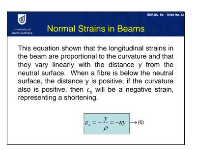
Equation 6 shows that the longitudinal strains in the beam are proportional to the curvature and that they vary linearly with the distance y from the neutral surface. When a fibre is below the neutral surface, the distance y is positive; if the curvature also is positive, then strain will be a negative strain, representing a shortening. Normal strain in linear function means normal stress is also a linear function, based on Hookes law.
