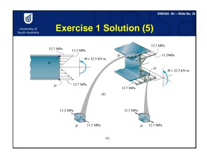
You can see the stress distribution for the I shape cross section in three dimensional view here, in figure d. The compressive normal stress cube at point B (the junction of the web and the flange) is equal to 11.2 Mega Pascals, as shown in figure e. The tensile normal stress cube at point D (the bottom most point) is equal to 12.7 Mega Pascals, as shown in figure e.
