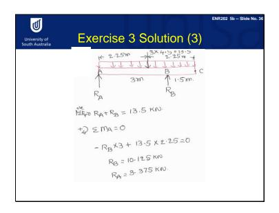
We have covered how to calculate reaction forces for an overhang beam (look back at lecture 4b, slide 27 if you need to). You have to use the equilibrium equation to calculate reaction forces. The first equilibrium equation is that all forces in a vertical direction are equal to zero. A second equilibrium equation is that all forces moment about point A equal zero. The answer is that the reaction force at support point A is 3.375 kilo Newtons and at support point B is 10.125 kilo Newton.
