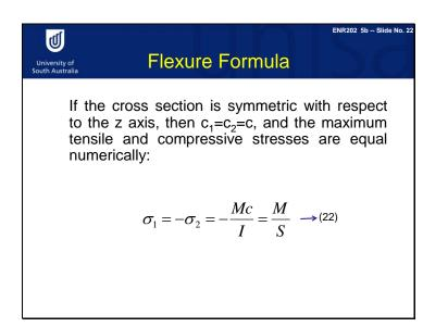
If we have a double symmetric cross section with C1 equal to C2, we can consider that S1 equals S2. Finally, we have sigma1 equals sigma2, as shown in equation 22.
