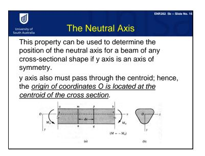
This property can be used to determine the position of the neutral axis for a beam of any cross-sectional shape if the y axis is an axis of symmetry, as shown in figure b. The y axis also must pass through the centroid point. Therefore, the origin of coordinates O is located at the centroid of the cross section.
