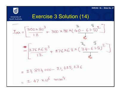
Try to calculate the moment of inertia about the x-x axis of the channel cross section by using the negative area principle, and then compare your answer to ours below.
