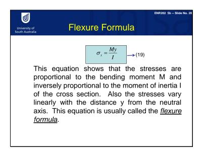
Equation 19 is the flexure formula. This equation shows that the stresses are proportional to the bending moment M and inversely proportional to the moment of inertia I of the cross section. Also, the stresses vary linearly with the distance y from the neutral axis.
