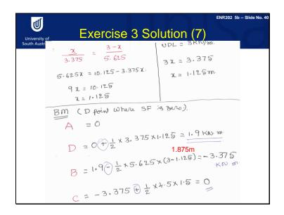
You can also calculate the distance 'x'; that is, the distance between points A and D where the shear force is zero, based on a similar triangle as shown in the calculations. Once we know the shear force diagram, we can draw the bending moment diagram based on shear force diagram. Start with the left end and then go back to the right end. We have 3 important points, A,B and C.
