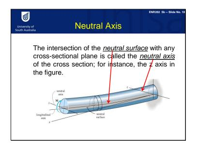
The intersection of the neutral surface with any cross section plane is called the neutral axis. For example, we have an s-s neutral surface, and we have this cross section in the beam. The z-line is a neutral axis as shown in the figure. In a neutral axis, we don't have any longitudinal deformation, we don't have any normal or normal stress.
