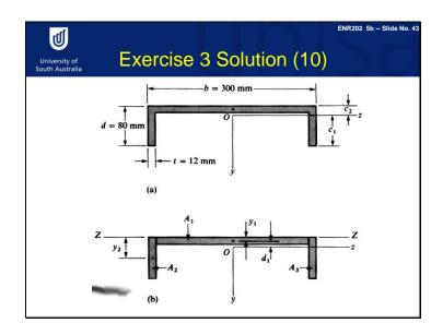
The cross section of the over hang beam is a channel section. You need to calculate the centroid and the moment of inertia for this channel section. The dimensions of the channel section are shown in figure a. You then need to find the centroid axis.
