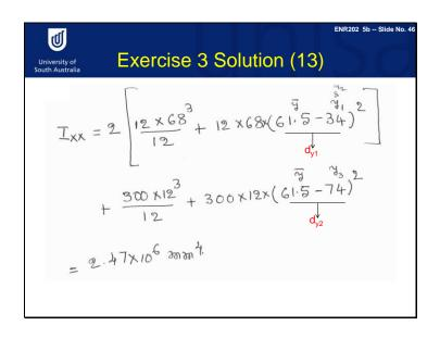
Now try to calculate the moment of inertia about the x-x axis of the channel cross section, and then compare your answer to our below.
