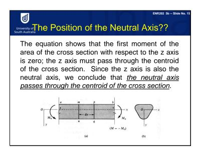
Equation 9 shows that the first moment of the area of the cross section with respect to the z axis is zero; the z axis must pass through the centroid of the cross section (that is, point O) as shown in figure b. Since the z axis is also the neutral axis, we conclude that the neutral axis passes through the centroid of the cross section, as shown in figure b.
