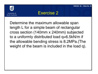
Now try this exercise. A simply supported beam with a rectangular cross section of 140 millimeters width and 240 millimeters depth is subjected to a uniformly distributed load 'q' of 6.5 kilo Newtons per meter. You need to calculate the maximum allowable span length 'L' if the allowable bending stress is 8.2 Mega Pascals. Assume that the weight of the beam is included in the uniform distributed load 'q'. The solution is on the next two slides.
