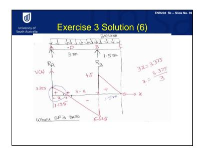
Connect all the values at important points, and we get shear force diagram as shown in the figure. We recommend you that draw shear force diagram on your own and check it against this figure.
