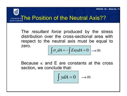
We can determine the position of neutral axis through analysing the normal force on the beam section.
