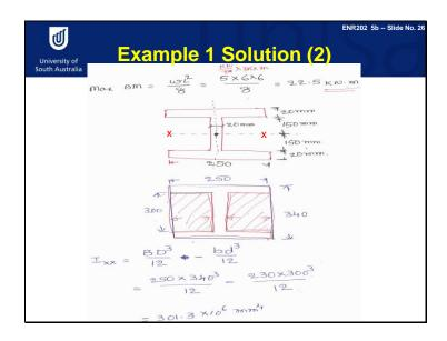
The maximum bending moment is equal to a uniform distributed load of 5 kilo Newton per meter times 6 meters times 6 meters divided by 8, which is equal to 22.5 kilo Newton Meters.
