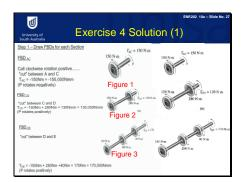
First, draw the Free Body Diagram for each section. We have 3 sections: AC, CD and DE. In the AC section, you cut the shaft between point A and point C, and draw the free body diagram as shown in figure 1. Apply the equilibrium equation and you will get the torque in section AC as being equal to 150 Newton meters. Due to TAC P, the point at gear A rotates negatively, so this torque sign is negative.
