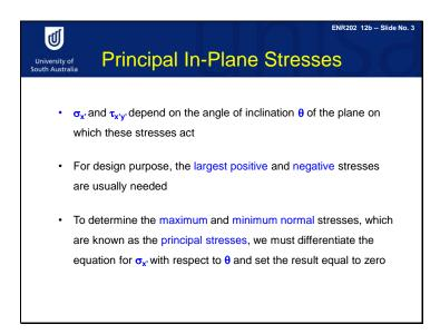
normal stress sigma x dash and shear stress tou x dash y dash depend on the angle of inclination theta of the plane on which we interested on these stresses. In engineering, you need to find largest positive stress and largest negative stress for design purpose.
