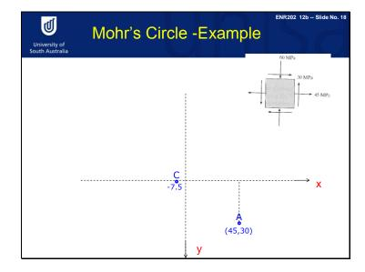
Third, you need to locate point A. the point A have the coordinates sigma x on x-axis and tou xy on y-axis. These sigma x and tou xy as shown in the right edge of the element called x face. On right edge of this element have normal stress is positive 45 Mega Pascals and positive shear stress 30 Mega Pascals. The coordinates of A is 45,30 as shown in the figure.
