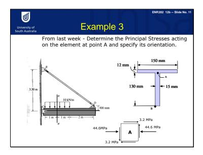
Do you remember this problem? We calculated normal stress and shear stress at points A and B in lecture 11b of example 3. I recommend you that go back to example 3 of lecture 11b and understand very well. We continue same thing from that problem to determine principal stresses at points A and B as shown in the bottom figure. We also need to determine the orientation of principal stress plane at point A.
