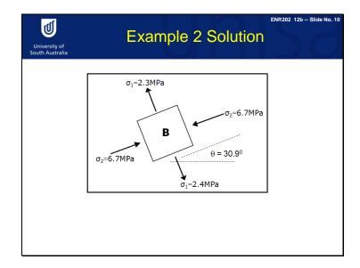
Can you have a look at this figure. We rotate the state of stress at point B 30.9 degrees in anti clock wise direction to get principal stress plane. And you can see maximum and minimum principal stresses as shown in the figure. As I said, we don't have any shear stresses in principal planes.
