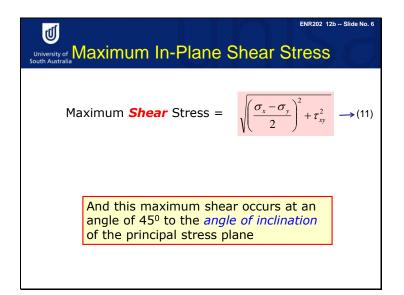
The maximum in plane shear stress equal to square root of sum of square root of sigma x minus sigma y divided by 2 and square of 'tou xy' as shown in the equation 11. If you want to know maximum shear stress plane, you just add 45 degree to the angle of inclination of the principal stress plane that is 'theta p' as explained in previous slide.
