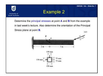
Do you remember this problem? We calculated normal stress and shear stress at points A and B in lecture 11b of example 1. I recommend you that go back to example 1 of lecture 11b and understand very well. We continue same thing from that problem to determine principal stresses at points A and B as shown in the bottom figure. We also need to determine the orientation of principal stress plane at point B.
