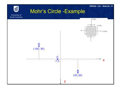
Fourth, you need to locate point G. the point G have the coordinates sigma y on xaxis and tou xy on y-axis. These sigma y and tou xy as shown in the top edge of the element called y face.
