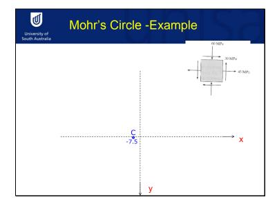
Second we need to locate the centre of circle that is average normal stress. The average normal stress is sigma x plus sigma y divided by 2. sigma x equal 45 Mega Pascals, sigma y equal minus 60 Mega Pascals. The average normal stress equal to plus 45 minus 60 divided by 2 equal to minus 7.5 Mega Pascals. Therefore, the centre point C should be negative side of x axis as shown in the figure.
