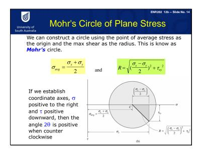
We use Mohr's circle to find magnitude and direction of principal stress and maximum shear stress. We can construct a circle using the point of average normal stress is sigma x plus sigma y divided by 2 as the origin of circle and maximum shear stress as the radius of circle. This circle known as Mohr's circle.
