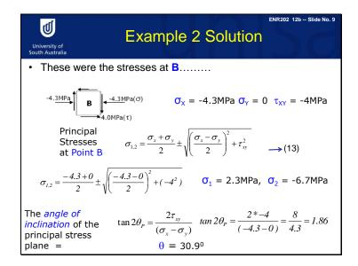
The state of stress at point B as shown in the figure that compressive normal stress in x plane is negative 4.3 Mega Pascals, and we don't have any normal stress in y plane that means sigma y equal to zero, and shear stress at right edge of element 4 Mega Pascals acting downward direction that means 'tou xy' equal to negative 4 Mega Pascals.
