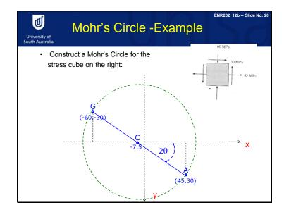
Fifth, connect the points A, C and G. This line forms the diameter of the Mohr's circle for this stress element. Draw Mohr circle with C point as centre of circle and A or G as radius of circle. Finally we have Mohr circle at this state of stress. Why we draw Mohr circle. Do you remember that.
