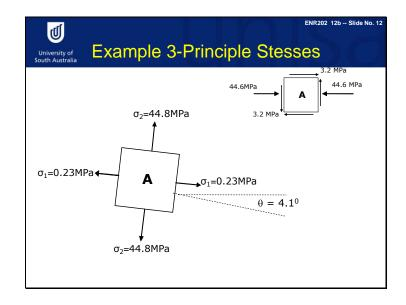
The state of stress at point A as shown in the figure that compressive normal stress in x plane is negative 44.6 Mega Pascals, and we don't have any normal stress in y plane that means sigma y equal to zero, and shear stress at right edge of element 3.2 Mega Pascals acting upward direction that means 'tou xy' equal to positive 3.2 Mega Pascals.
