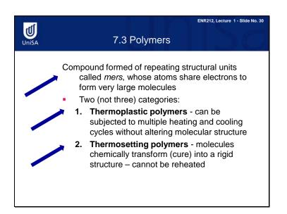
Polymers are entangled long chain molecules. They are divided into thermoplastics and thermosets, depending on their behaviour in increasing temperature. If temperature is increased, thermoplastic can be melted, molded and reused. However, thermosets can not be melted, reused and recycled because of the chemical bonding between chains of thermosets.
