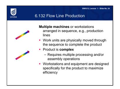
Flow line production contains Multiple machines or workstations arranged in sequence. The products in a flow line production are complex.
