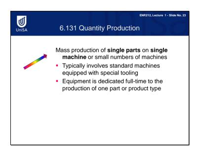
Quantity production refers to Mass production of single parts on single machine or small numbers of machines. The main feature of quantity production is single parts or single products.
