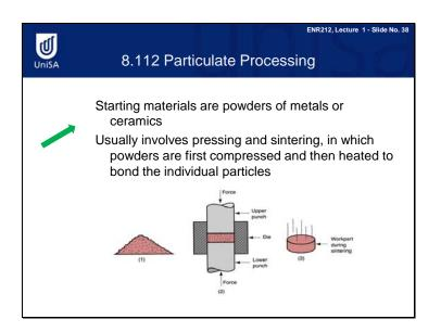
Particulate processing usually involves pressing and sintering, in which powders are first compressed and then heated to bond the individual particles.
