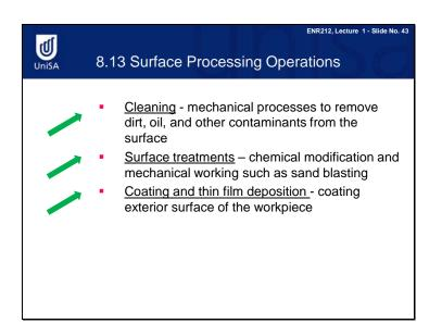
Surface processing operations include cleaning, surface treatment, and coating and thin film deposition.
