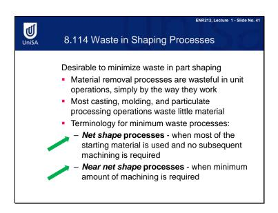
In shaping processes, it is desireable to minimize waste. Depending on the quantity of waste produced, shaping processes are classified into net shape processes and near net shape processes. Net shape processes produce no waste. Near net shape processes produce a little waste.
