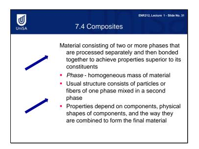
In plain words, a composite is a mixture of different materials. If a composite is a mixture of two materials, we call it a two-phase composite.
