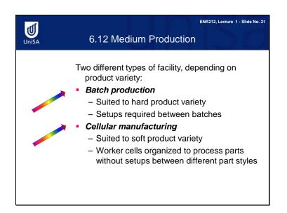
There are two type of facilities for medium production: batch production facilities and cellular manufacturing facilities. Batch production suit hard product varieties, where there is a big difference in the products. It needs setups between batches. Cellular manufacturing facility suit soft product varieties. There is no set up needed between different batches.
