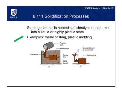
In solidification processes, the starting material is heated sufficiently to transform it into a liquid or highly plastic state
