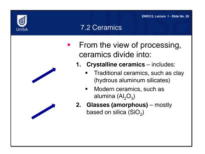
Ceramics are compounds of metallic and nonmetallic elements. Depending on the crystallinity, they are classified into crystalline ceramics and amorphous ceramics. Crystalline ceramics are often stronger and tougher than amorphous ceramics. However, amorphous ceramics are normally transparent. That is the advantage of amorphous ceramics.
