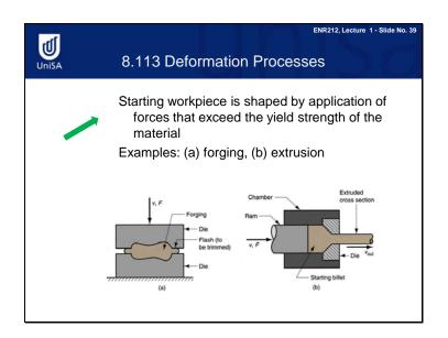
In deformation processes, the starting workpiece is shaped by application of forces that exceed the yield strength of the material.
