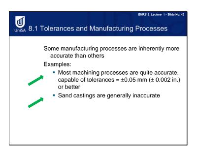
Tolerance is an important element of mechanical design. Most machining processes are accurate, although they may produce waste. Lower tolerances means higher costs. Sand casting is inaccurate, but produces minimum waste. Near net waste processes have a higher tolerance.
