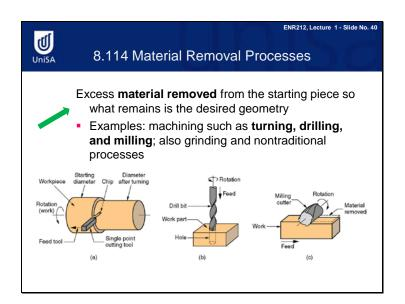
In material removal processes, excess materials are removed from the starting part to obtain a desired geometry.
