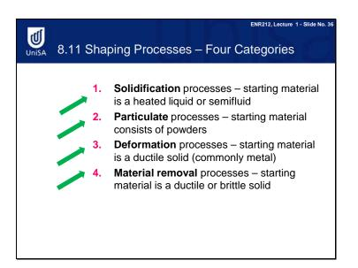
There are four categories of shaping processes. Solidification processes start with a material which is a heated liquid or semifluid. In Particulate processes, the starting material consists of powders. In deformation processes, the starting material is a ductile solid. In this unit, we refer to a ductile metal. In material removal processes, the starting material is a ductile or brittle solid.
