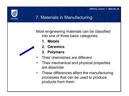
In general, there are three types of materials in manufacturing. They are metals, ceramics and polymers. These materials are structurally different, and thus have completely different physical and mechanical properties. So which of these three - metals, ceramics and polymers - is the toughest? Which one is stiffest? And which one has the highest specific strength?
