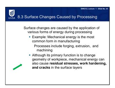
In manufacturing, surface changes are caused by the application of various forms of energy during processing. Mechanical energy is the most common form, such as drilling, forging, extrusion and machining. However, the mechanical energy can cause residual stresses and cracks in the surface layers, which need to be avoided.
