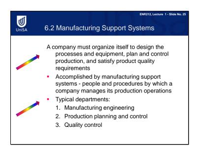
To operate the facilities efficiently, a company must organize itself to design the processes and equipment, plan and control production, and satisfy product quality requirements. Manufacturing support systems contain the following types of departments: manufacturing engineering, production planning, and control and quality control.
