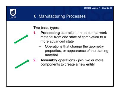
Manufacturing processes include processing operations and assembly operations. Processing operations transform a work material from one state of completion to a more advanced state. The purpose of a processing operation is to enhance properties or improve the appearance of the starting material. Assembly operations join two or more components to create a new entity.
