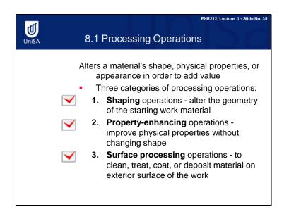
Processing operations consist of three branches: shaping operations, property enhancing operations, and surface processing operations. These are the focus of this unit.
