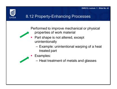
Property enhancing processes are operations to improve the mechanical or physical properties of a material without changing the material geometry, such as the mechanical properties and the stiffness of a metal. A typical example is heat treatment of metals and glasses, such as anealling.
