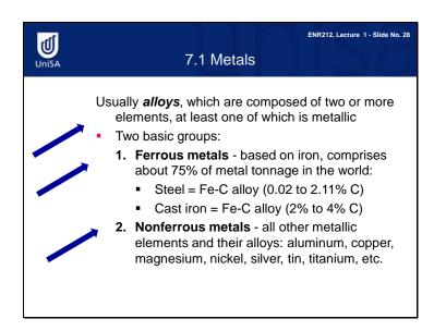
Metals are usually alloys, which are composed of two or more elements, at least one of which is metallic. Metals are classified as ferrous metals and nonferrous metals. Ferrous metals are based on iron. They comprise about 75% of metal tonnage in the world. Nonferrous metals refer to all other metallic elements and their alloys: aluminum, copper, magnesium, nickel, silver, tin, and titanium.
