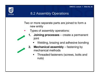
Assembly operations contain joining processes and mechanical assembly. Joining processes create a permanent joint. On the other hand, mechanical assembly is really just fastening by mechanical methods. It is not permanent.
