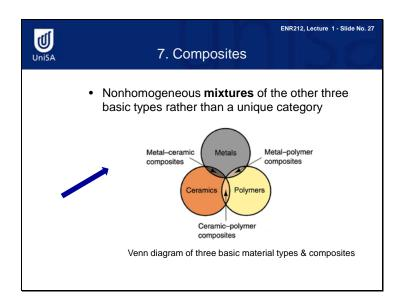
The three types of composites are shown in this figure, where you can see mixtures of different materials. The purpose of making composites is to obtain averaged properties.
