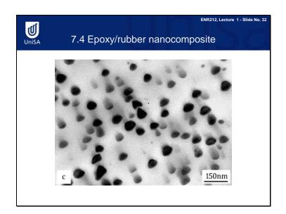
This photograph represents the morphology of epoxy rubber composites. Epoxy takes ninety volume %. Rubber only takes ten volume %. These black particles represent rubber particles. Epoxy is brittle, while rubber is very ductile. So mixing ductile rubber particles with epoxy certainly toughens epoxy.
