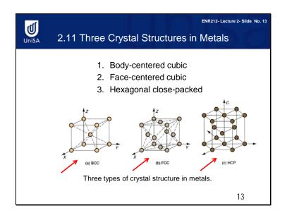
There are three crystal structures for metals: body-centered cubic structure, face-centered cubic structure and hexagonal close-packed structure.
