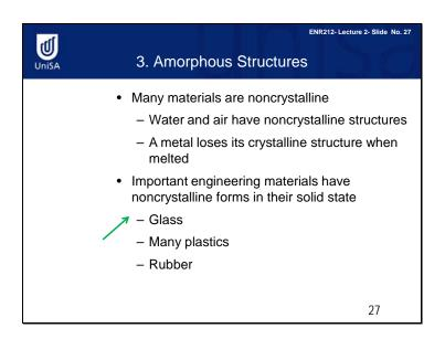
Metals have crystalline structures. However, polymers are different. Some are crystalline, some are semi-crystalline and some are just amorphous. Amorphous materials should be transparent (such as glass).
