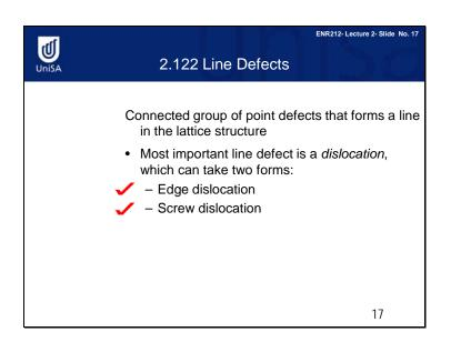
Line defects are connected point defects that form a line in the lattice. Line defects are classified into edge dislocations and screw dislocations.
