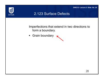
Surface defects are actually grain boundaries. The grain boundaries are just areas between crystals, between the grains of metals.
