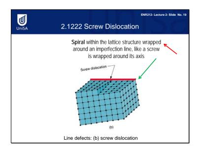
A screw dislocation is a spiral in the lattice structure which is wrapped around an imperfection line, as you can see in this image. The red line represents an imperfection line.
