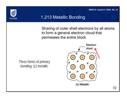
In metallic materials, each atom contributes at least an electron, so there are a great many electrons in a metal. These electrons have complete freedom. That is, one electron is able to move from one atom to another. Therefore, metallic bonding is not directional. This explains why metallic materials are electrically and thermally conductive and why metals are normally stronger than organic materials such as wood, which comprises covalent bonding.
