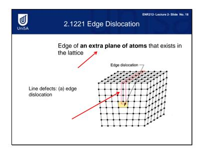
An edge dislocation is the edge of an extra plane of atoms that exists in the lattice. In this image, the area included in the red rectangle represents an edge dislocation.
