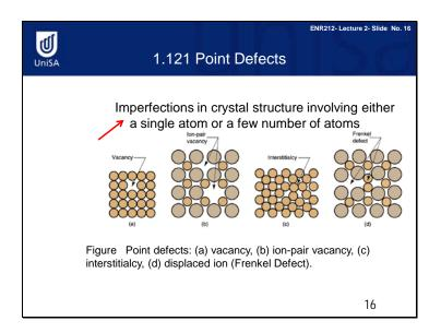
Point defects are imperfections in the crystal structure of metals, in which only one or a few atoms are missing.
