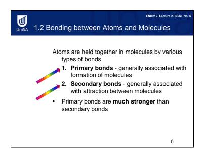
There are two levels of interaction in materials. Primary bonds exist between atoms. Secondary bonds exist between molecules. In general, primary bonds are much stronger than secondary bonds. This explains why metals generally have higher absolute strength than polymers.
