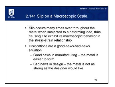
However, dislocation or defects are a double-edge sword. Dislocations are desired in manufacturing, because they reduce the manufacturing cost. However, dislocations are not good in material design, because dislocation reduces the strength of materials.
