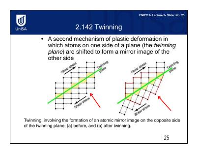
Slip is the first mechanism of plastic deformation. The second mechanism is twinning. The left image shows a lattice before plastic deformation. The green line represents a twinning plane. You can see the lattice geometry above the plane is similar to the lattice below the plane. Now look at the second image. After the shear deformation, the geometry of the lattice above the plane is different to the lattice below the plane. This phenomenon is called twinning.
