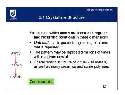
In a crystalline structure, the atoms are arranged at regular and recurring positions. That is, the atoms in a crystalline structure are disordered. Atoms are combined into unit cells. Unit cells are combined to produce crystals. The size of atoms is around 0.1 to 0.13 nanometers. The average size of unit cells is around 0.4 to 0.6 nanometers. The size of crystals range from nanometers to millimeters.
