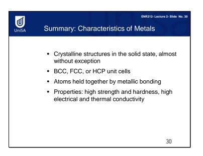
Metals are crystalline in their solid state. Metal atoms are held together by metallic bonding. There are a large number of free electrons, and this sets the high strength, high stiffness and high electrical and thermal conductivity of metal.
