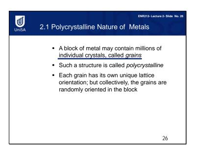
Metals are crystalline materials. Metals contain crystals. These crystals are also called grains. Here are two questions for you.
