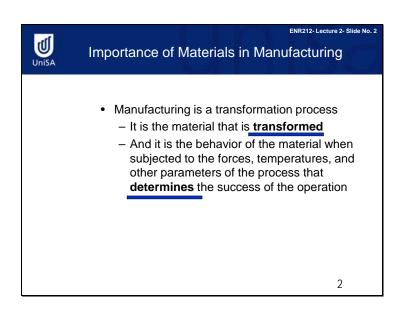
Materials are of great importance in manufacturing for two reasons. First, the aim of manufacturing is to transform materials from one state to another more advanced state with increased value. Second, it is the material properties that determine the manufacturing processes, such as the set up of machines.
