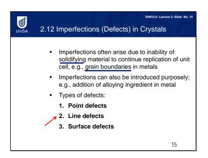
During solidification processes, imperfection or defects in crystals of metals are produced when the temperature is reduced from melting temperature to room temperature. An example of defects is grain boundaries. As we have discussed, grain boundaries are the area between crystals and grains. There are three types of defects: point defects, line defects and surface defects. Surface defects are actually grain boundaries.
