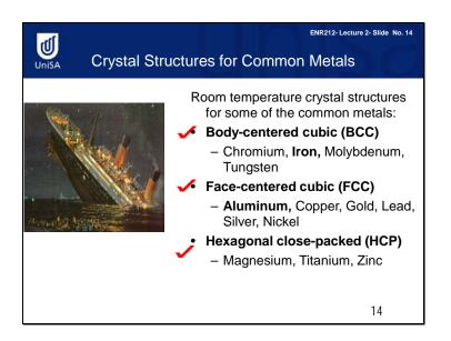
Body-centered cubic materials, such as iron, have very good strength at room temperature, but their fracture toughness at low temperature is poor. Do you remember the movie 'Titanic'. It was about a ship which sank, leading to the loss of 2000 lives. It sank because it was made of iron, which has low toughness at low temperatures in icy water.
