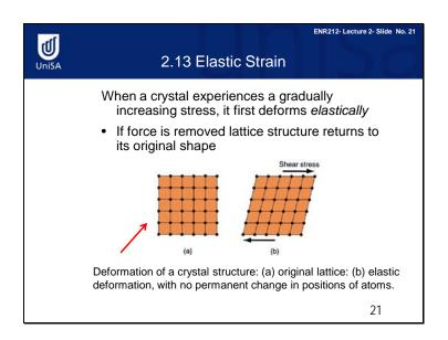
There are two types of deformation of materials: elastic deformation and plastic deformation. An example of elastic deformation is the elongation of a rubber band. Plastic deformation examples include the fracture of ductile thermal plastics.
