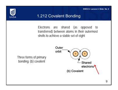
Shared electrons are involved in covalent bonding. As you see in this figure, a pair of electrons is shared by two atoms. This means the covalent bonding is directional. Therefore, covalent bonding such as in wood is not electrically and thermally conductive.
