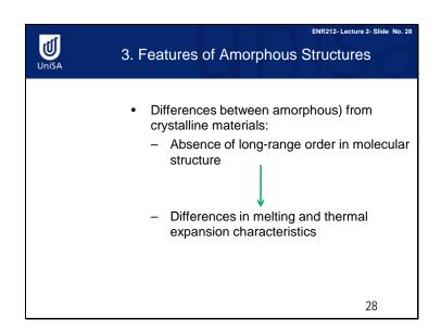
We have looked at crystalline structure. In crystalline structures, the atoms are arranged at regular and recurring positions. In amorphous structures, there is no long-range order in molecular structure. This means that there are huge differences in melting and thermal expansion characteristics.
