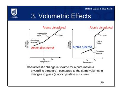
An amorphous material shows very different thermal behaviour to a crystalline material. For example, with temperature changes, the volume change for an amorphous material is different to the volume change for a crystalline material.
