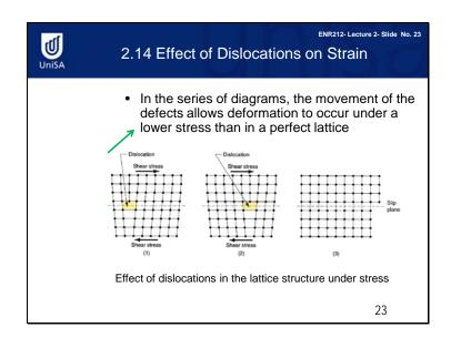
As advised before, dislocations and defects are important in manufacturing. Defects and dislocations are desired, because more dislocations means lower yield strength, which means lower cutting force is needed in manufacturing. This saves energy and time.
