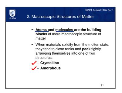
The building blocks of materials include atoms and molecules. Atoms are the building blocks of metals, while molecules are the building blocks of polymers. Materials are classified into crystalline and amorphous, according to how the atoms arrange themselves.
