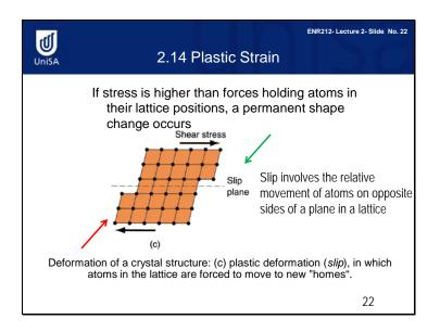
Plastic strain is similar to plastic deformation. The deformation produced is not recoverable. This image shows plastic strain in a lattice. Under increasing shear stress, plastic deformation occurs. This plastic deformation is permanent and not recoverable. This kind of deformation is called slip. What is slip? Slip involves the relative movement of atoms on opposite sides of a plane in a lattice.
