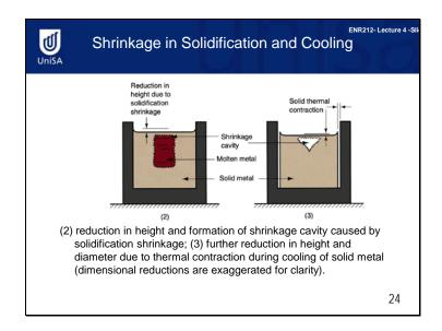
Solidification contraction occurs from figure 1 to figure 2. Because the molten metal solidifies inward towards the top centre, with obvious shrinkage, metal flows from the top centre towards the surround region. Therefore, there is always a void in the final region to freeze, as shown in Figure 3. This void is created by the absence of metal, and is called a pipe. Once solidified, the casting experiences further contraction in height and diameter.
