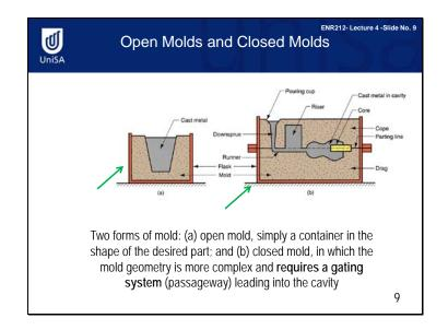
To accomplish a casting operation, the metal is first heated to a temperature which is high enough to completely transform it into a liquid state. It is then poured, or otherwise directed, into the cavity of the mould. In an open mould, the liquid metal is simply poured in until it fills the cavity. In a closed mould, a passageway, called the gating system, lets the molten metal flow from outside the mould into the cavity. Slide 10
