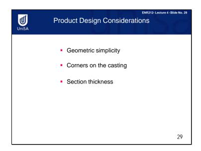
Although casting can be used to produce complex part geometries, simplifying the part design usually improves castability. Sharp corners and angles should be avoided, since they are sources of stress concentrations and may cause hot tearing and cracks. Section thicknesses should be uniform in order to avoid shrinkage cavities.
