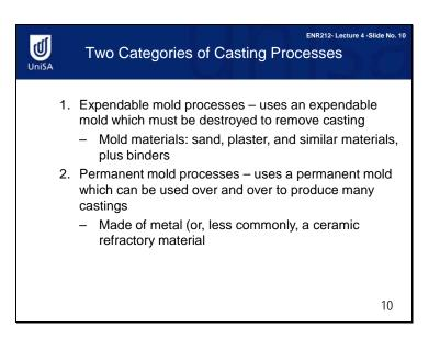
There are two categories of casting processes: expendable mould processes and permanent mould processes.
