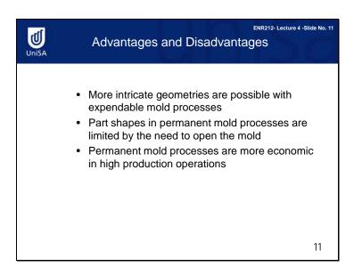
If we compare expandable processes with permanent mould processes, we can see that more sophisticated casting geometries are generally made with the expendable mould processes.
