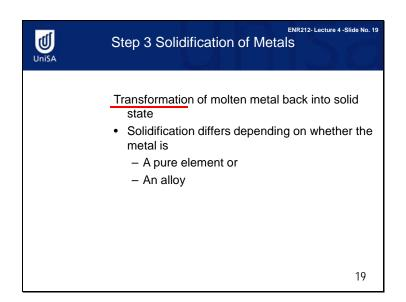
Solidification involves the transformation of the molten metal back into the solid state. The solidification process differs depending on whether the metal is a pure element or an alloy.
