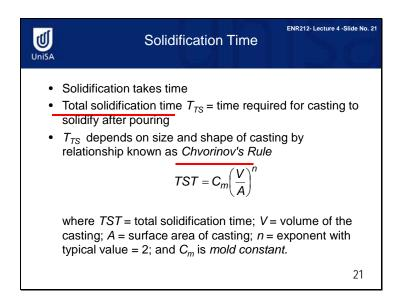
The total solidification time is the time required for the casting to solidify after pouring. This time is dependent on the size and shape of the casting by an empirical relationship known as Chvorinov's rule.
