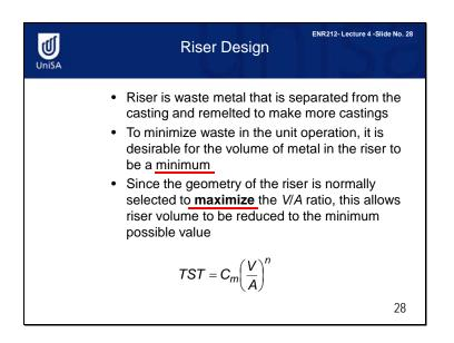
The riser is waste metal that is separated from the casting and remelted to make more castings. To minimize waste in the unit operation, it is desirable for there to be a minimum volume of metal in the riser. Since the geometry of the riser is normally selected to maximize the V over A ratio, this allows riser volume to be reduced to the minimum possible value.
