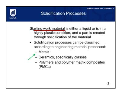
In a solidification process, the starting work material is either a liquid or is in a highly plastic condition, and a part is created through solidification of the material. According to the materials processed, the solidification processes can be classified into: metal casting for metals, ceramics solidification processes, and thermal plastic moulding for polymers.
