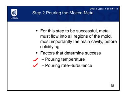
After heating, the metal is ready for pouring. The introduction of molten metal into the mould, including its flow through the gating system and into the cavity, is a critical step in the casting process. For this step to be successful, the metal must flow into all regions of the mould before solidifying. The factors which affect the pouring operation include the pouring temperature, the pouring rate, and the turbulence.
