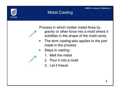
Casting is a process in which molten metal flows by gravity or by other types of force into a mould, where it solidifies in the shape of the mould cavity. The term casting is also applied to the part that is made by this process. The principle of casting seems simple: just melt the metal, pour it into a mould, and let it cool and solidify. However, there are many factors and variables that must be considered in order to accomplish a successful casting operation.
