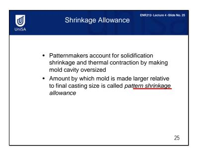
Pattern-makers account for solidification shrinkage and thermal contraction by making the mould cavities oversized. The amount by which the mould must be made larger relative to the final casting size is called the pattern shrinkage allowance.
