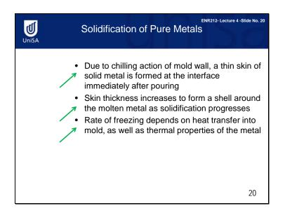
When molten metal is chilled, a thin skin of solid metal is initially formed at the interface immediately after pouring.
