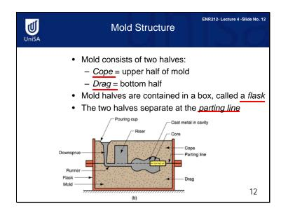
A mould consists of two halves: the cope and the drag. The cope is the upper half of the mould, and the drag is the bottom half.
