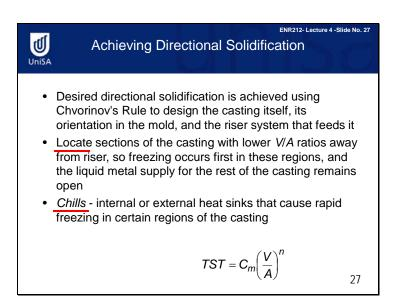
Chvorinov's rule can be used to achieve direction solidification by mould design. For example, we can locate parts of the casting with lower ratios away from the riser, so solidification occurs first in these regions, and there is still molten metal supply for the rest of the parts. We use chills to achieve rapid freezing.
