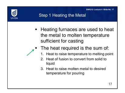
Heating furnaces of various kinds are used to heat the metal to a molten temperature sufficient for casting. The heat energy required is the sum of the following three energies: first, the heat to raise the temperature to the melting point, second, the heat of fusion to convert it from solid to liquid, and third, the heat to raise the molten metal to the desired temperature for pouring.
