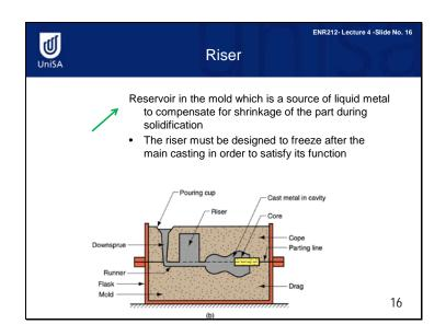
Now, as we have discussed, shrinkage can be a serious problem. Any casting in which shrinkage is significant requires a riser connected to the main cavity, in addition to the gating system. The riser is a reservoir in the mould that serves as a source of liquid metal for the casting, to compensate for shrinkage during solidification. Here are three questions to research for interest:
