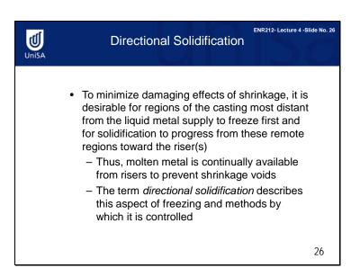
In simple words, directional solidification is a metal solidification in which the molten metal is controlled to solidify from the remote regions toward the risers.
