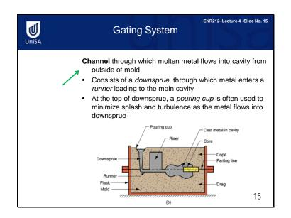
The gating system in a casting mold is the channel, or network of channels, by which molten metal flows into the cavity from outside the mould.
