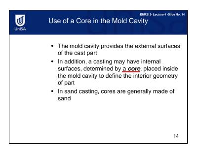
The cavity in the mould provides the external surfaces of the cast part. In addition, a casting may have internal surfaces. These surfaces are determined by means of a core, which is placed inside the mould cavity to define the interior geometry of the part. In sand casting, cores are generally made of sand, although other materials can be used, such as metals, plaster, and ceramics.
