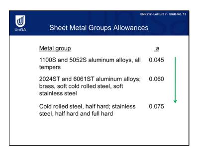
Different metals have different cutting allowances. In general, the more brittle a metal, the more clearance it needs in shearing.
