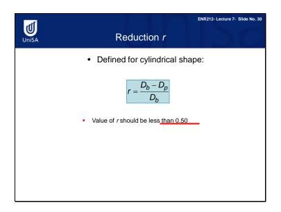
The reduction for a drawing operation can be obtained from this equation. The reduction is equal to the blank diameter minus the punch diameter, all divided by the blank diameter. The value of the reduction should be less than 0.5 for the operation to be feasible.
