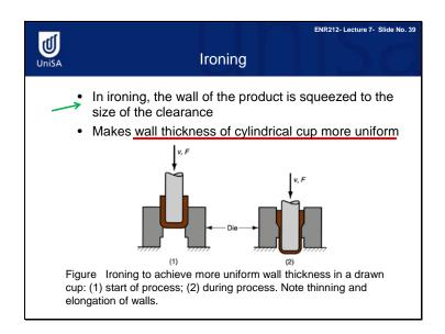
There is sometimes a problem with the deep drawing process. Because the flange is compressed by the squeezing action between the punch and the die, its perimeter becomes smaller as it is drawn towards the die opening, and the wall thickness obtained is often not uniform. Ironing is a process which doesn't have this problem, because the wall of the product is squeezed to the size of the clearance, so the wall thickness is more uniform than in deep drawing.
