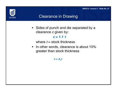
The clearance in drawing is about 10% greater than the stock thickness.
