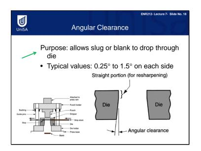
In order for the slug or blank to drop through the die, the die opening must have an angular clearance of 0.25<sup>2</sup> to 1.5<sup>2</sup> on each side.
