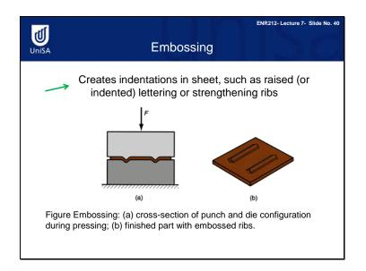
Embossing is a forming operation used to create indentations in the sheet. It involves some stretching and thinning of the metal.
