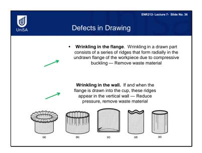
There are five major defects in drawing. The first is wrinkling in the flange. When we talk of wrinkling in a drawn part, we mean a series of ridges that form radially in the undrawn flange of the workpiece, due to compressive buckling. This defect can be fixed up by removing waste material. The second defect is wrinkling in the wall. This can be cured by reducing pressure and removing waste material.
