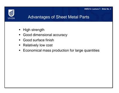
Sheet-metal parts are generally characterized by high strength, good dimensional accuracy, good surface finish, and relatively low cost. If you think back to earlier lectures, you will realize that these features are actually the advantages of cold working, because sheet metal working is often conducted at room temperature (which is cold working).
