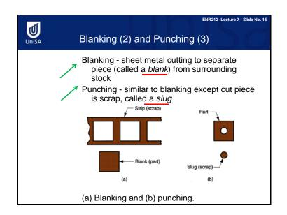
Blanking involves cutting sheet metal along a straight line in a single step, to separate a piece from the surrounding stock. The part that is cut out is the desired product, and is called a blank. Punching is similar to blanking, except that the cut piece is scrap, and is called a slug. The remaining stock is the desired product.
