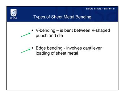
In V-bending, a sheet metal is bent between a V-shaped punch and die. Edge bending involves cantilever loading of the sheet metal.
