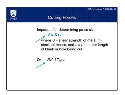
Accurate estimation of the cutting force is important, because it is this force which determines the size of the press needed. The cutting force 'F' in sheet metalworking can be determined by this equation, where S = shear strength of metal; t = stock thickness, and L = perimeter length of blank or hole being cut. Since the testing of shear strength is much more difficult than the tensile strength testing, we need the second equation to estimate a cutting force.
