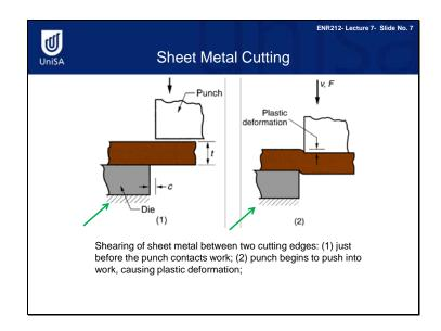
Cutting of sheet metal is accomplished using two sharp cutting edges. The shearing action is shown in these four figures. The upper cutting edge is called the punch and the lower is called the die. In Figure 1, the punch sweeps down past the die while the die is stationary. In Figure 2, as the punch begins to push into the metal sheet, plastic deformation occurs in the surfaces of the sheet.
