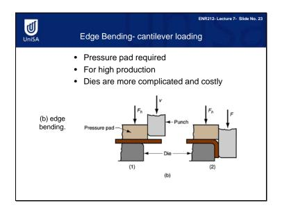
As we have stated, edge bending involves the cantilever loading of a sheet metal. So in edge bending, a pressure pad is used to apply a force to hold the work part against the die, while the punch forces the part to yield and bend over the edge of the die. Because of the pressure pad, the dies are more complicated and costly than V-dies, and are generally used for high-production work.
