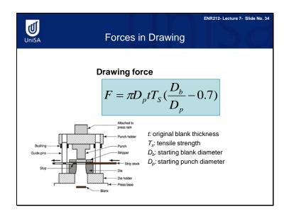
You can roughly estimate the drawing force required to perform a given operation by the formula given on this slide.
