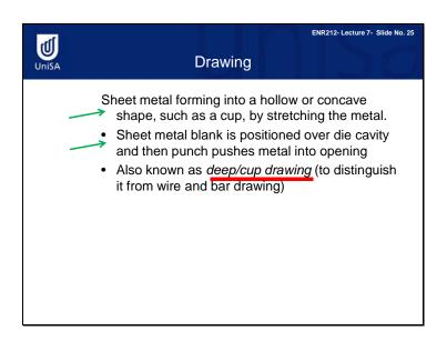
Drawing refers to the forming of a flat metal sheet into a hollow or concave shape, such as a cup, by stretching the metal. The sheet metal blank is positioned by the blankholder over the die cavity and then the punch pushes metal into the opening.
