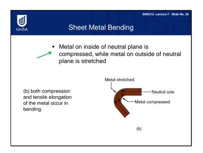
During the bending operation, the metal on the inside of the neutral plane is compressed, while the metal on the outside of the neutral plane is stretched.
