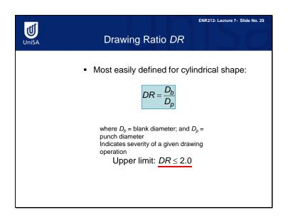
For a cylindrical shape, the drawing ratio is defined as the ratio of blank diameter to punch diameter. The drawing ratio should be larger than 2.0 for the operation to be feasible. The equation for calculating the drawing ratio is DR = blank diameter divided by punch diameter.
