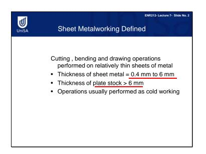
We have already looked at rolling. If you remember, rolling is a metal bulk deformation process. In a typical rolling, the thickness of a metal plate is reduced by two rotating mills. The starting work material in rolling is a metal plate. On the other hand, sheet metalworking operations are performed on relatively thin sheets of metal. Typically, the sheets are between 0.4 mm and 6 mm thick, while plate stock is usually thicker than 6mm.
