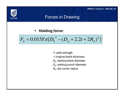
The holding force in drawing is given by this equation. In some of the assessment activities for this unit, you will be asked to calculate the holding force and compare your calculation with the measured value.
