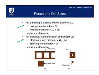
The determination of punch and die sizes in punching and blanking is tricky. (You can assume that this will be one of the tasks which are part of quizzes and the exam.) For punching, if a round hole of diameter D h is requested, then the hole die diameter is equal to D h plus 2c, where C represents clearance. For blanking, if a round blank of diameter D b is requested, then the blanking punch diameter equals D b minus 2c.
