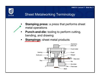
A stamping press is a press that performs sheet metal operations. In sheet metal working, the punch-and-die tool is often used to perform cutting, bending, and drawing operations. The products are called stampings.
