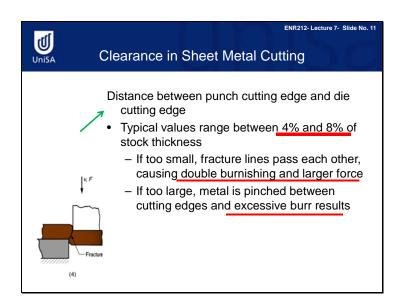
The clearance in sheet metal cutting refers to the distance between the punch cutting edge and die cutting edge. Typical clearance values range between 4% and 8% of stock thickness. If the clearance is too small, the fracture lines pass each other, causing double burnishing and larger cutting forces. If they are too large, the metal is pinched between cutting edges and you will get excessive burr results.
