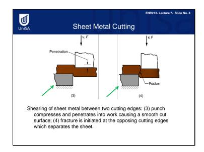
In Figure 3, as the punch continues to move downward, penetration occurs, in which the punch compresses the sheet and cuts into the metal. This penetration zone is generally about one-third the thickness of the sheet. In Figure 4, as the punch continues to travel into the work, fractures initiate and grow in the workpiece at the two cutting edges. If the clearance between the punch and die is correct, the two fracture planes meet, resulting in a clean separation of the work into two pieces.
