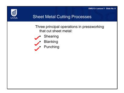
There are three principal operations used to cut metal in pressworking: shearing, blanking, and punching. Shearing involves using two cutting edges along a straight line to separate a metal sheet. Blanking involves cutting sheet metal along a closed outline in a single step to separate a piece from the surrounding stock. Punching is similar to blanking, except the cut piece is scrap.
