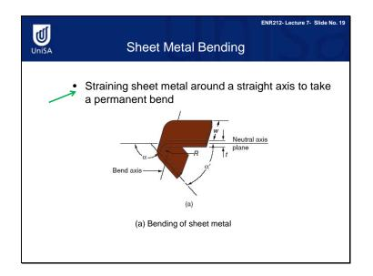
Bending in sheet metalwork is defined as straining of a metal sheet to take a permanent angle along a straight axis.
