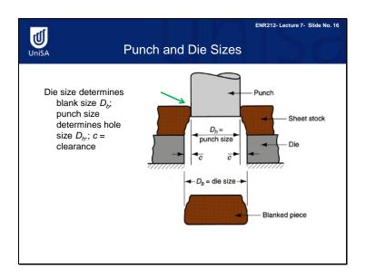
This figure shows you a hole produced by a metal cutting process. Note that the hole has a non-uniform diameter. Therefore, blanking and punching processes have different ways to determine the diameter of the punch and die.
