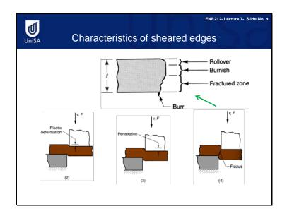
A cut piece of metal consists of four zones: rollover, burnish, fractured zone and burr. The size of the burr can be minimized by adjusting the gap between the punch and the die.
