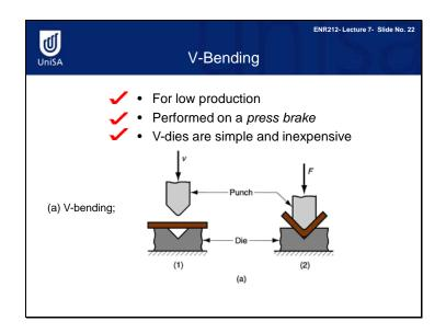
V-bending is generally used for low-production operations. It is often performed on a press brake, and the associated V-dies are relatively simple and inexpensive.
