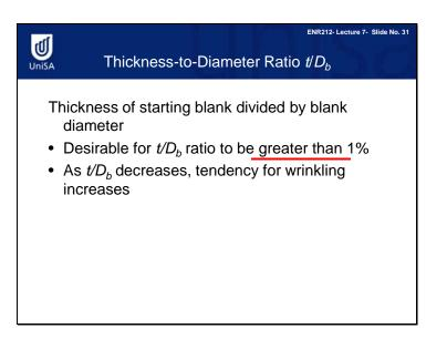
In deep drawing, the thickness-to-diameter ratio of the starting piece must be greater than 1.0 for the operation to be feasible. The thickness to diameter ratio is calculated by dividing the thickness of the starting blank by the blank diameter.
