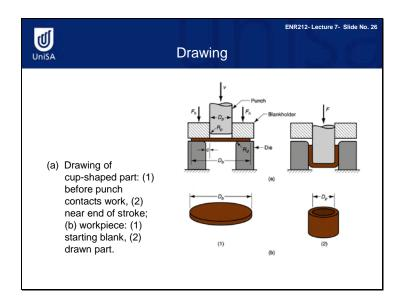
This slide shows you a drawing process. You can see the metal flow is a characteristic of drawing.
