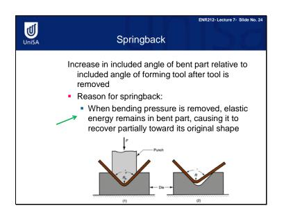
After the punch is removed, the angle increases due to elastic deformation. The increase in the angle is called springback. Springback is illustrated in this figure.
