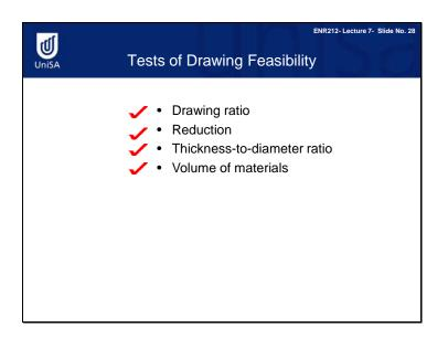
The drawing feasibility of a metal piece is determined by these four conditions: the drawing ratio, reduction, thickness-to-diameter ratio, and the volume of materials.
