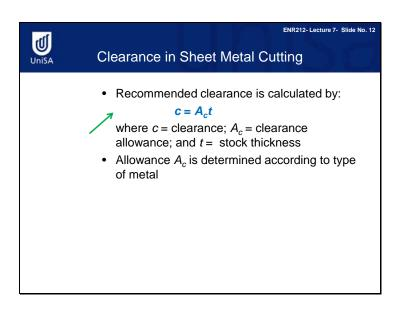
You use the formula above to calculate the recommended clearance, where c equals the clearance, A C equals the clearance allowance, and t equals the stock thickness. Clearance allowance is determined according to the type of metal.
