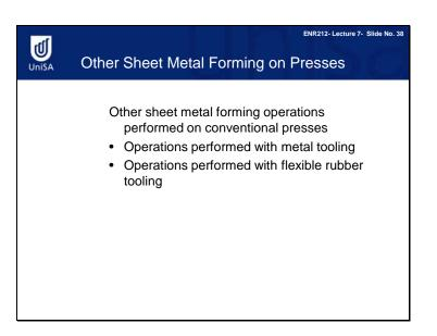
We have learnt about the three major types of sheet metalworking, which are cutting, bending and drawing. However, there are other sheet metal processes and some of these operations are performed with metal tooling, in the same way as the three major types. There are also operations performed with flexible rubber tooling. (Rubber is a type of polymer.)
