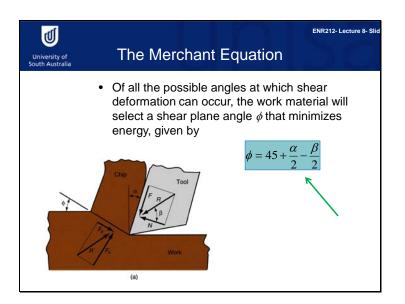
One of the most important equations in metal cutting is the merchant equation. This equation states that the shear plane angle is 45 plus rake angle divided by 2 minus friction angle divided by 2.
