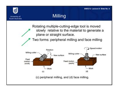
In milling, a rotating tool with multiple cutting edges is moved slowly across the material to generate a plane or straight surface. There are two forms of milling, peripheral milling and face milling.
