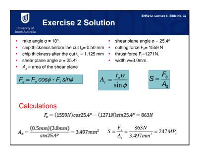
To do this, we need to determine the shear force Fs and the shear stress S. You can see the three equations which you need, and the actual calculations, in this slide.
