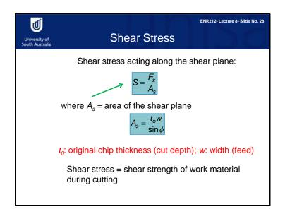
In past lectures, we have looked at what stress and engineering stress are. Stress is equal to the load divided by the original cross-sectional area. So, what is shear stress? Shear stress is defined as a stress acting along the shear plane. Shear stress is equal to the load divided by the area of the shear plane.
