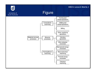
The Shaping operations include material removal processes. The common feature of these processes is that they remove material from a starting workpiece so that the remaining part has the desired geometry. Material removal processes include machining processes, abrasive processes and nontraditional machining processes. \*In machining processes, materials are removed by a sharp cutting tool (for example, through turning, milling and drilling).
