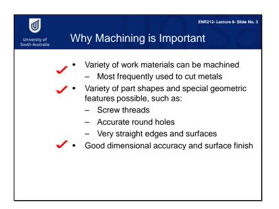
Machining is important because it has three main strengths. It can be applied to a wide variety of work materials, including metals, plastics, thermosets, composites and even ceramics. In fact, it is the most frequently used method to cut materials. It can be used to create any special geometries, such as screw threads. Finally, it can produce good dimensional accuracy and surface finish.
