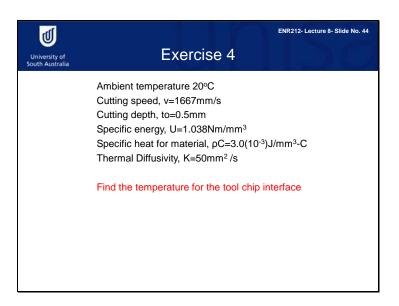
Now, you can use the Nathan's equation to predict the cutting temperature in this example. You have been given the ambient temperature, the cutting speed and depth, the specific energy, the specific heat for the material and the thermal diffusivity. Find the temperature rise for the tool chip interface. The solution is on the next slide.
