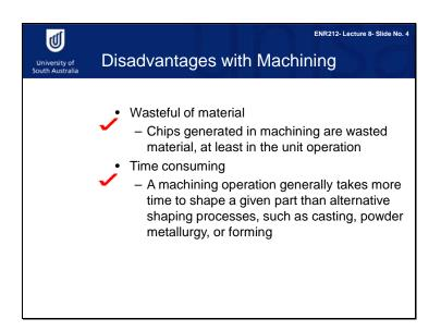
However, machining has two weaknesses. First, it is inherently wasteful of materials, because it removes materials from a starting workpiece. Second, a machining operation generally takes more time to shape a given part than alternative shaping processes such as casting or moulding.
