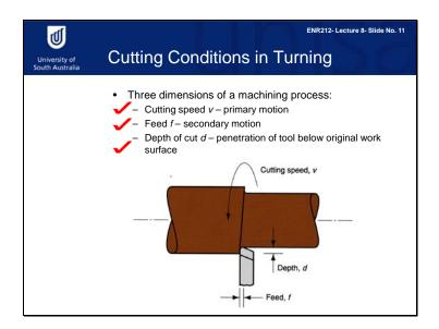
We have looked at two types of relative motions in a turning operation, speed motion and feed motion. This slide shows you the three dimensions which must be considered in a machining process. They are the cutting motion, the feed motion and the depth of the cut.
