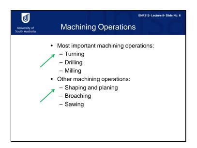
There are three most commonly used machining operations. They are turning, drilling and milling. However, other machining operations include shaping and planing, broaching, and sawing.
