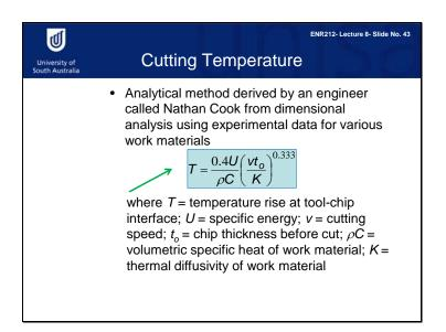
It is important to control the cutting temperature. Nathan Cook developed an equation for predicting cutting temperature.
