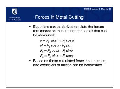
Cutting force and thrust force are used to calculate shear force, friction force, and normal force to friction, by these four equations.
