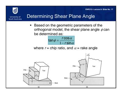
In a chip formation process, the shear plane angle is the angle between the horizontal plane and the shear plane. It is calculated by this equation: Tan angle is equal to chip ratio cosine rake angle divided by 1 minus chip ratio sine rake angle.
