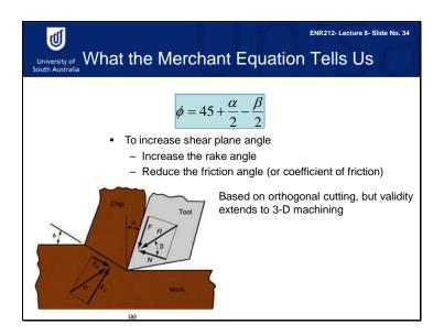
What does the merchant equation tell us? It tells us that to increase shear plane angle, we need to increase the rake angle, while reducing the friction angle.
