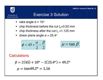
You can see the two equations which you need for this problem in this slide. The coefficient of friction between the tool and chip is tan friction angle. The friction angle can be derived by rearranging the Merchant equation, because you know the shear plane angle and the rake angle. The solution is that the friction angle is 49.2 degrees and the coefficient of friction is 1.16.
