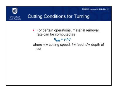
For most single-point tool operations, the material removal rate can be calculated using this equation. The Material Removal Rate is equal to the cutting speed multiplied by the feed multiplied by the depth of the cut.
