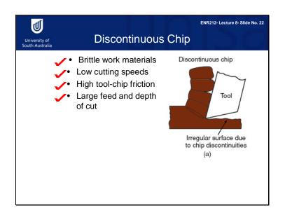
Discontinuous chips are produced by brittle materials, such as cast iron, at low cutting speeds. High tool-chip friction and large feed and depth of cut can cause this type of chip to form.
