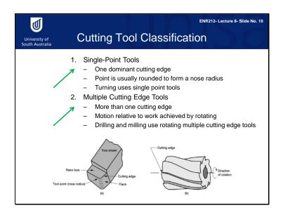
There are two basic classifications of cutting tools, single-point and multiple-cuttingedge. A single-point tool has one cutting edge and is used for operations such as turning. A multiple-cutting-edge tool has more than one cutting edge and usually achieves its motion relative to the workpiece by rotating. These tools are used for drilling and milling operations.
