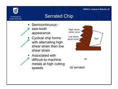
Serrated chips possess a saw-tooth appearance. They are the result of alternating high shear strain and then low shear strain. This type of chip is most closely associated with certain difficult-to-machine metals being machined at high cutting speeds, such as titanium alloys.
