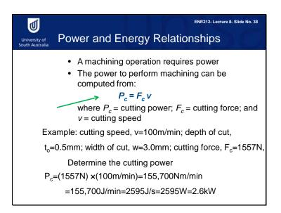
A machining operation requires power, and you will need to work out the amount of power you require for specific operations. The equation for this is cutting power equals cutting force multiplied by cutting speed. For example, if we have an operation with a cutting speed of 100 meters per minute, and a cutting force of 1557 Newtons, then the power needed is 155, 700 Newton meters per minute, which equals 2.6 kilo Watts.
