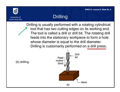
Drilling is a machining process which is usually performed with a rotating cylindrical tool that has two cutting edges on its working end. The tool is called a drill or drill bit. The rotating drill feeds into the stationary workpiece to form a hole whose diameter is equal to the drill diameter. Drilling is customarily performed on a drill press. This figure shows you a drilling process.
