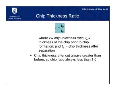
To calculate the chip thickness ratio, divide the chip thickness before chip formation by the chip thickness after separation. The thickness after the cutting is always greater than the thickness before, so the chip ratio is always less than 1.0.
