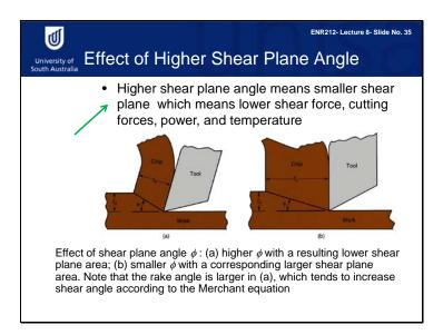
This slide shows you the relationship between the shear plane angle and the cutting force. A higher shear plane angle means a smaller shear plane, which means lower shear force, cutting forces, power, and temperature.
