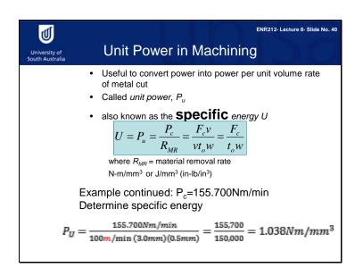
The unit power is the amount of power required to remove per unit volume of cut metal. It is calculated by dividing the cutting power by the material removal rate. To continue the previous example, if the cutting power is 155.7 Nm per minute, and the material removal rate is 100 meters per minute, then the Unit power is 1.038 Nm per cubic mm.
