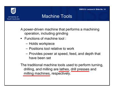
Machine tools are just the machines that accomplish the material removal processes. The machine tool for turning is called a lathe, and the machine tool for drilling is called a drill press. The machine tool for milling is called a milling machine.
