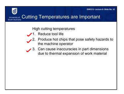
High cutting temperatures are not good at all, for a number of reasons. They reduce tool life, they produce hot chips that pose safety hazards to the machine operator, and they can cause inaccuracies in part dimensions, due to the thermal expansion of work material.
