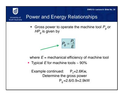
The gross power needed to operate the machine tool is calculated by dividing cutting power by the mechanical efficiency of the machine tool, which is typically 90%. So, to continue the last example, if we divide the cutting power by 90%, we get a gross power of 2.9 kilo Watts.
