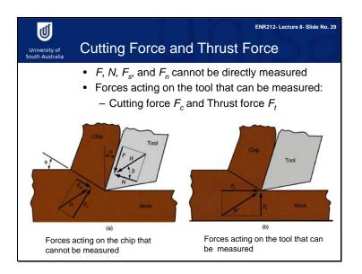
When a cutting tool is forced into a working material, two forces are needed, and these are measurable. The cutting force is in the direction of cutting, the same direction as the cutting speed. The thrust force is perpendicular to the cutting force and is associated with the chip thickness before the cut.
