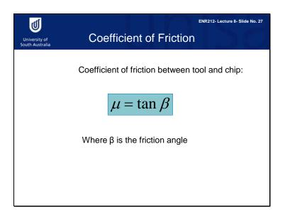
The friction between tool and chip is important. The coefficient of friction between the tool and chip is tan friction angle.
