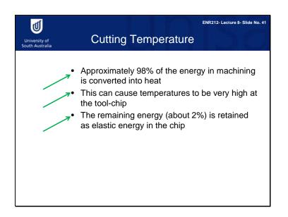
Approximately 98% of the energy in machining is converted into heat. This can cause very high temperatures at the tool-chip. The remaining energy (about 2%) is retained as elastic energy in the chip.
