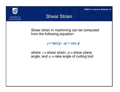
We have looked at strain in previous lectures. Strain is relative to the deformation of a material. Shear strain is relative to the deformation of material in shearing. The shear strain in machining is calculated by tan shear plane angle minus rake angle, plus cos shear plane angle.
