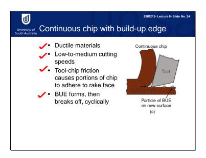
When ductile materials are being machined at low-to-medium cutting speeds, friction between the tool and the chip tends to cause portions of the work material to adhere to the rake face of the tool near the cutting edge. This can form a continuous chip with a built up edge (BUE). The formation of a BUE is cyclical; it forms and grows, then becomes unstable and breaks off.
