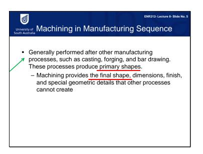
The weaknesses of machining can be overcome to some extent if the machining is performed after other manufacturing processes, such as casting or bulk deformation. These processes create the primary shapes of the starting workpiece, and these primary shapes are subsequently machined to produce the final geometry, dimensions, and finish.
