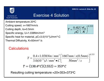
Nathan Cook's equation is given here. You should have used this equation to work out that the cutting temperature rise is 353 degrees Celsius. Given the ambient temperature of 20 degrees, this means that the resultant cutting temperature is 373 degrees Celsius.
