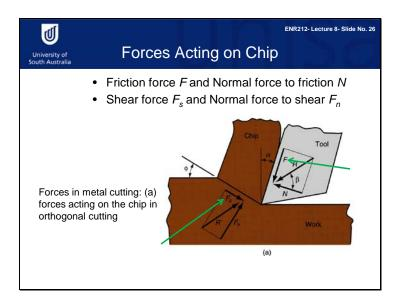
As shown in this figure, there are four forces in total in a typical machining process. The friction force is the frictional force which resists the flow of the chip along the rake face of the tool. The normal force to friction is perpendicular to the friction force. The shear force is the force that causes shear deformation to occur in the shear plane, and the normal force to shear is perpendicular to the shear force.
