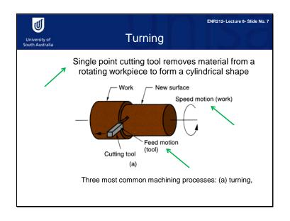
In turning, a cutting tool with a single cutting edge is used to remove material from a rotating workpiece to generate a cylindrical shape. There are two types of relative motion. The first is speed motion provided by the rotating workpiece, and the second is feed motion, achieved by moving the cutting tool slowly in a direction parallel to the axis of rotation of the workpiece.
