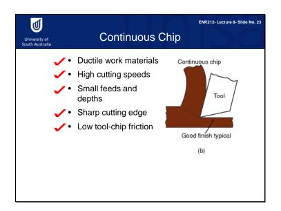
Continuous chips are formed by ductile materials at high speeds with relatively small feeds and depth. They are caused by sharp cutting edges on the tools and low tool-chip friction.
