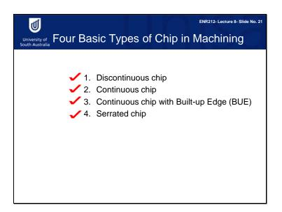
A chip is produced by shear deformation when a single-edge cutting tool is forced into a rotating part. Depending on the type of material being machined and the cutting conditions of the operation, four basic types of chips can be distinguished: discontinuous chip, continuous chip, continuous chip with a built-up edge, and serrated chip.
