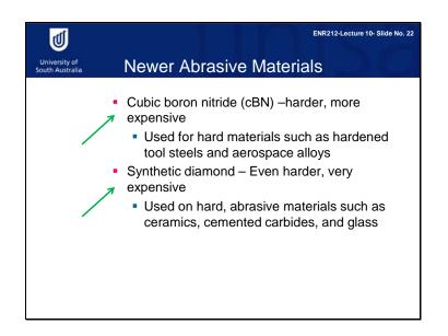
Cubic boron nitride is harder and more expensive than the first two materials. It is used for hard materials, such as hardened tool steels and aerospace alloys. The last abrasion material is synthetic diamond. It is the hardest and the most expensive of the four materials. It is used on hard, abrasive materials such as ceramics, cemented carbides, and glass.
