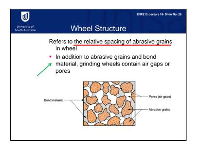
Wheel structure refers to the relative spacing of the abrasive grains in the wheel. This figure shows that a wheel structure includes bond material, pores and abrasive grains.
