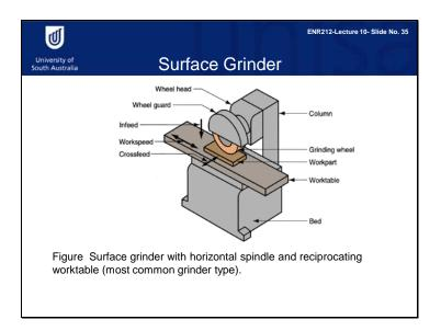
This figure shows you a surface grinder which has a reciprocating worktable and a horizontal spindle in the grinding wheel.
