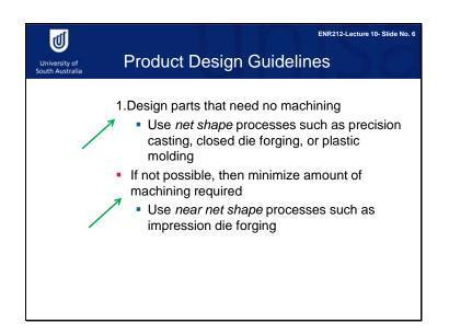
There are seven product design guidelines for conventional machining operations. First guideline. If possible, parts should be designed in a way that doesn't need machining. In general, products produced by using net shape processes such as precision casting, closed die forging, etc, cost less to produce. If machining cannot be avoided, then minimize the amount of machining required on the parts.
