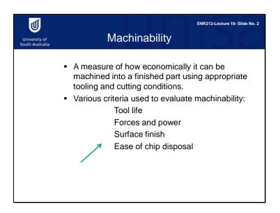
The properties of a work material have a significant influence on the machining operation of that material. These properties and other characteristics of the work material are often summarized in the term "machinability". The machinability of a material is a measure of how economically it can be machined into a part. Machinability is evaluated by the four criteria: tool life, forces and power, surface finish and ease of chip disposal.
