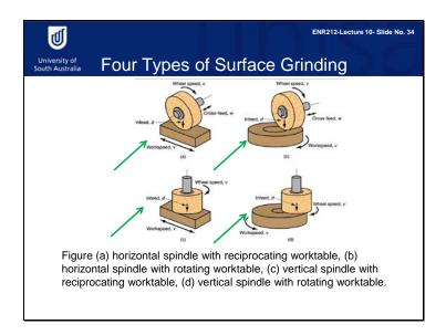
There are four types of surface grinding, depending on the relative motion between the worktable and the spindle of the grinding wheel. As you can see in figure a, this surface grinding machine has a horizontal spindle with a reciprocating worktable. In figure b, the grinding facility has a horizontal spindle with a rotating worktable. In figure c, the grinder has a vertical spindle with a reciprocating worktable. In figure d, the grinder has a vertical spindle with a rotating worktable.
