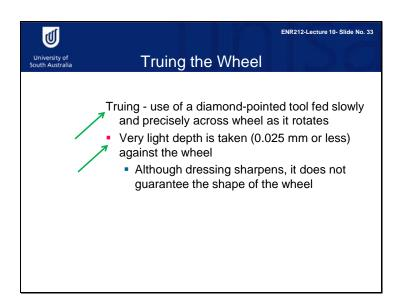
Dressing is a procedure to resharpen a worn grinding wheel. Truing is an alternative procedure. The procedure involves feeding a diamond-pointed tool slowly and precisely across the wheel as it rotates. Truing makes a very light depth (25um) against the wheel.
