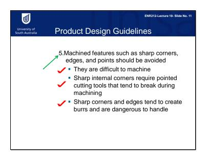
Fifth guideline. Machined features such as sharp corners, edges, and points should be avoided. There are three reasons for this: they are difficult to machine, they tend to break during machining, and they are a safety hazard.
