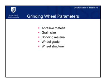
These abrasive particles and bonding material are the two ingredients, and the way they are fabricated determines the five basic parameters of a grinding wheel: abrasive material, grain size, bonding material, wheel grade, and wheel structure. Each of the parameters must be carefully selected to achieve the desired performance in an application.
