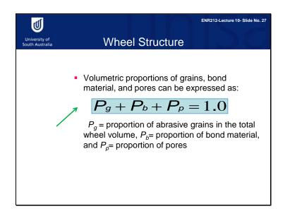
The volumetric proportions of grains, bond material, and pores can be expressed in this equation.
