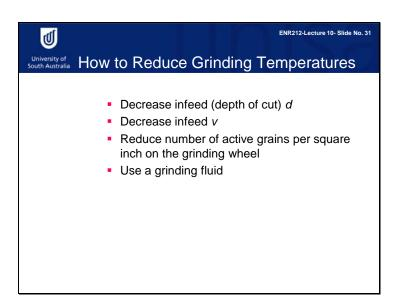
High grinding temperatures are harmful, but can be reduced. There are four ways to do this: decrease the infeed depth of cut, decrease the infeed, reduce the number of active grains per square inch on the grinding wheel, and use a grinding fluid. Of these methods, the most effective is using grinding fluid.
