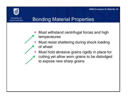
The bonding material holds the abrasive grains and establishes the shape and structural integrity of the grinding wheel. The bonding material must be able to withstand the centrifugal forces and high temperatures experienced by the grinding wheel. It must resist shattering in shock loading of the wheel. It must hold the abrasive grains rigidly in place to accomplish the cutting action while allowing worn grains to be dislodged so that new grains can be exposed. That is what we called friability.
