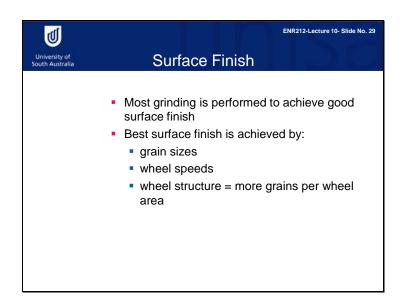
Most grinding is performed to achieve a surface finish that is superior to what can be accomplished with conventional machining.
