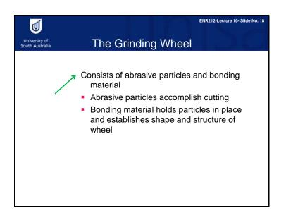
A grinding wheel consists of abrasive particles and bonding material. The role of the abrasive particles is to accomplish cutting, and the role of the bonding material is to hold the particles in place and to establish the shape and structure of the wheel.
