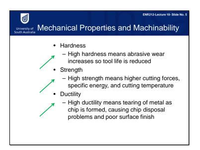
We know that the machinability of a material is determined by the mechanical properties of this material. To demonstrate good machinability, a material must possess moderate mechanical properties.
