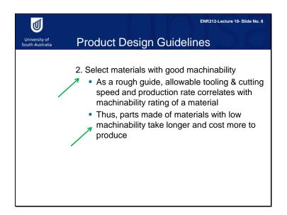
Second guideline. Select materials with good machinability, because the tooling and cutting conditions and production rate of a material correlate with the material's machinability. Parts made of materials with low machinability take longer and cost more to produce.
