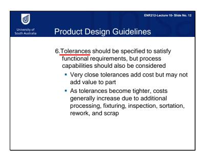
Sixth guideline. Machining is time consuming, but it provides good surface finish and close tolerances. We know that good surface finish and close tolerances are desirable in design, but that means a high manufacturing cost. Therefore, we need to evaluate the level of tolerance and surface finish needed by taking into account the end application of the product, the machining time and tool life.
