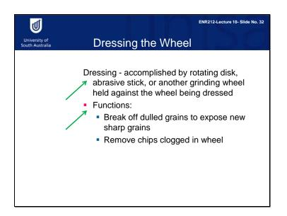
When a grinding wheel is worn, it is resharpened by dressing and truing. Dressing is accomplished by using a dressing tool. The tool can be a rotating disk or an abrasive stick, or another grinding wheel. Operating at high speed, the tool is held against the wheel to be dressed. The dressing breaks off dulled grains to expose new sharp grains and removes chips clogged in the wheel.
