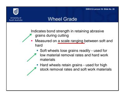
Wheel grade indicates the grinding wheel's bond strength in retaining the abrasive grains during cutting. The grade is measured on a scale that ranges between soft and hard. Soft wheels lose grains readily and are used for low material removal rates and hard work materials. Hard wheels retain grains and are used for high stock removal rates and soft work materials.
