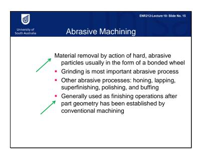
Abrasive machining processes use hard, abrasive particles (usually in the form of a bonded wheel) for material removal operations. Abrasive machining processes are generally used as finishing operations after the part geometry has been established by conventional machining operations.
