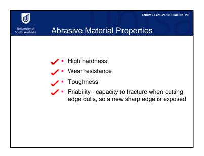
A grinding wheel consists of abrasive particles and bonding material. The desirable properties of the abrasive materials include high hardness, wear resistance, toughness and friability.
