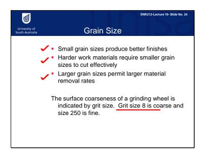
These materials are in the form of particles, and the grain size is the actual size of the materials. A smaller grain size produces better finish, and is more suitable for harder material, when it corresponds to lower removal rates. Grit size is a grinding product indicator. It is the opposite to grain size.
