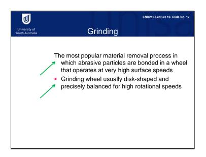
Grinding is the most popular abrasive machining process. In grinding, abrasive particles are bonded in a wheel that operates at very high surface speeds. Most grinding wheels have a disk-like shape and are precisely balanced for high rotational speed.
