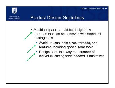
Fourth guideline. Machined parts should be designed with features that can be achieved with standard cutting tools. This means avoiding unusual hole sizes, threads, and features requiring special form tools. It is helpful to design a part in a way that minimizes the number of individual cutting tools. This often allows the part to be completed in one setup on a machining center with limited tool storage capacity.
