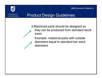
Third guideline. In order to minimize the amount of machining, the exterior dimensions of a part should be chosen to equal the standard stock size. For example, choose rotational parts with outside diameters that are equal to standard bar stock diameters.
