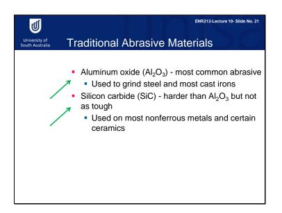
There are four important materials used for abrasion. The two traditional materials are aluminium oxide and silicon carbide. Aluminium oxide is the most commonly used. It is used for grinding steel and for most cast irons. Silicon carbide is harder than aluminium oxide but not as tough. Silicon carbide is used on most nonferrous metals and certain ceramics.
