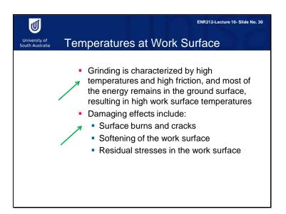
The grinding process is characterized by high temperatures and high friction. The high surface temperatures have several damaging effects: surface burns and cracks, softening of the work surface (like a polymer sample) and residual stresses in the work surface.
